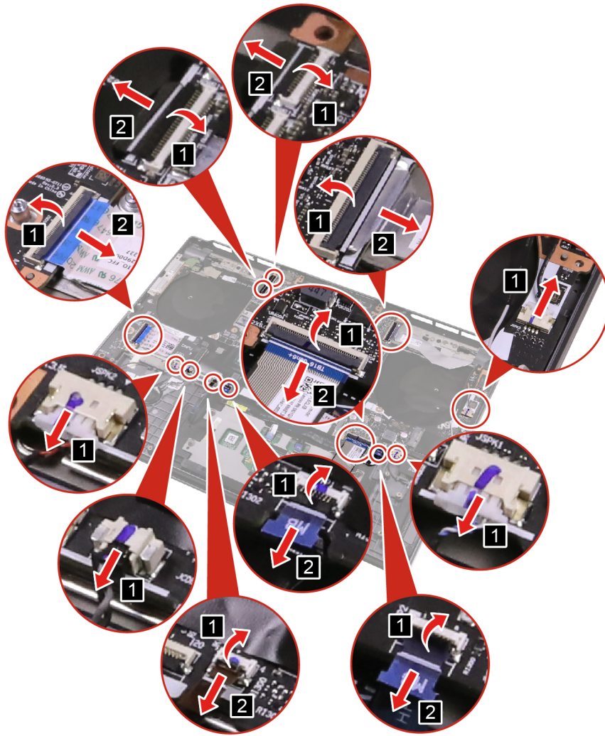
Figure 39. Disconnect all connections from the system board
