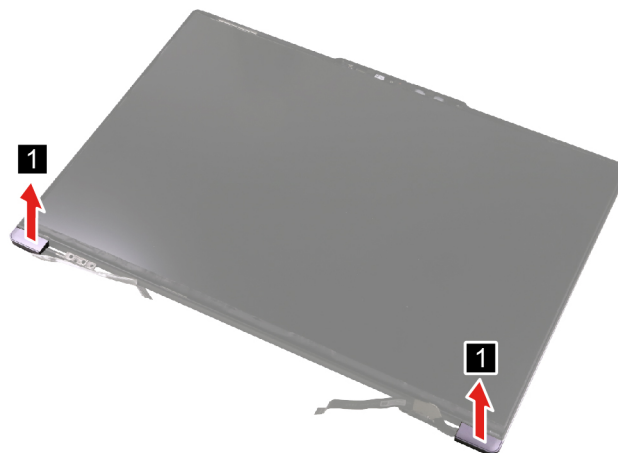
Figure 54. Remove the strip covers
