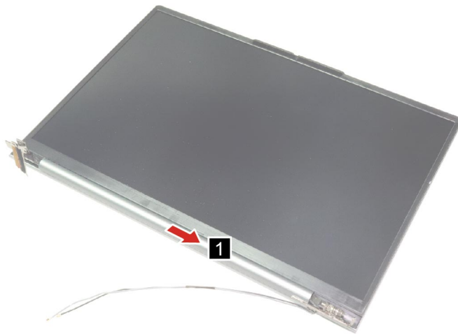
Figure 41. Remove the hinge cover
