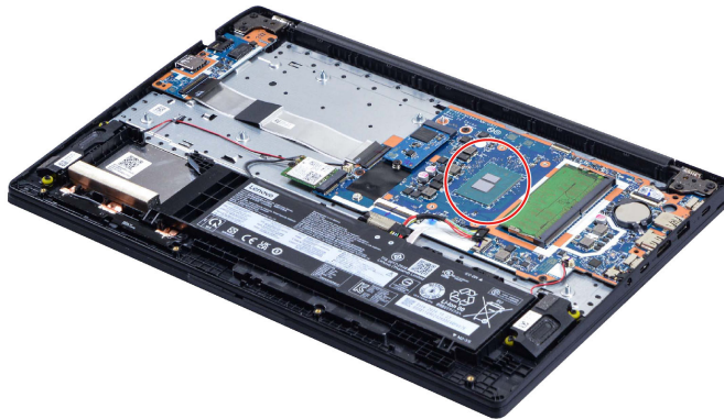
Figure 5. Areas on the system board where thermal interface materials are applied (15-inch models)
