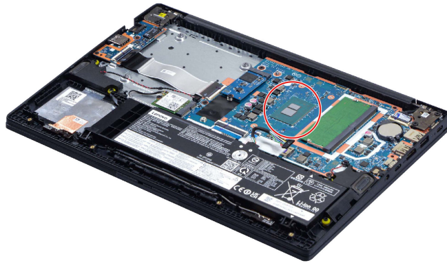
Figure 4. Areas on the system board where thermal interface materials are applied (14-inch models)
