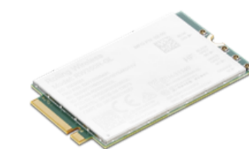
ThinkPad Rolling Wireless RW350 Sub6 5G WWAN Module for P16 G3 4XC1U10820
