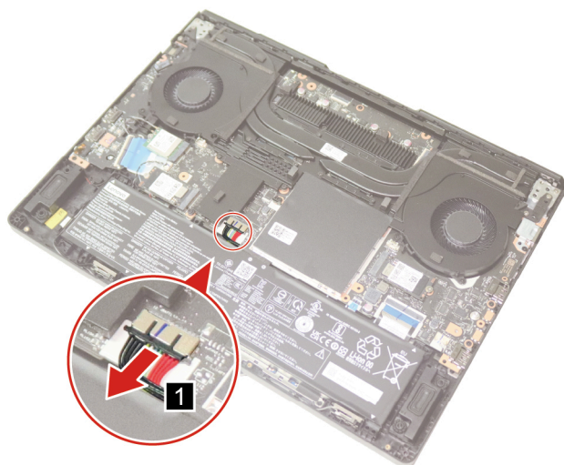
Figure 8. Disconnect the battery pack cable
