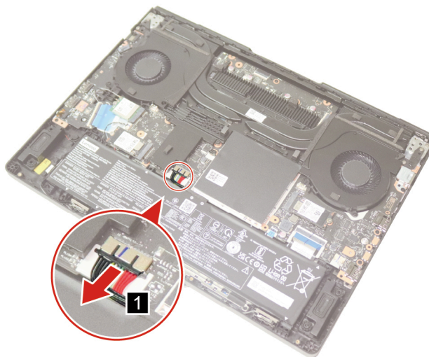
Figure 14. Disconnect the battery pack cable
