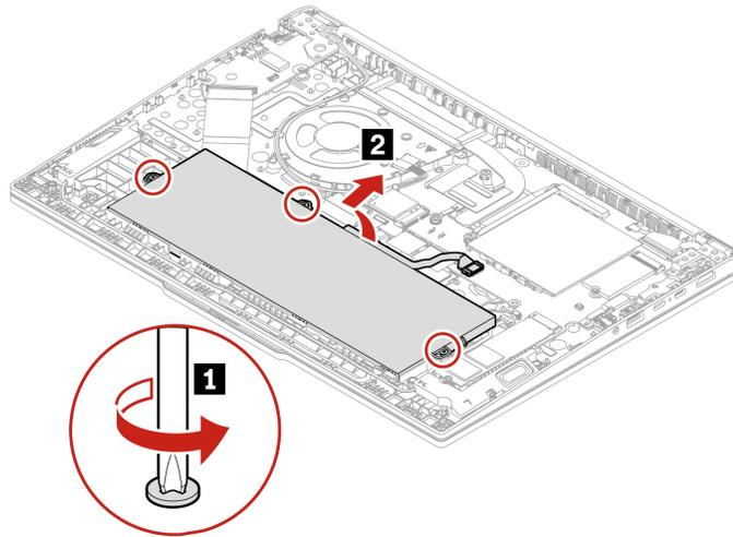
Step 2. Before installing the built-in battery, thoroughly check the battery compartment and ensure that there are no foreign or sharp objects that could cause damage to the battery.
