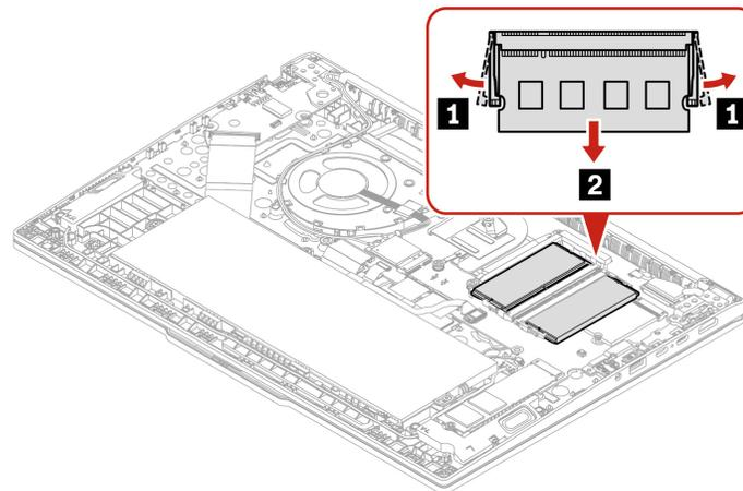
Step 2. Install the memory module as shown below.
