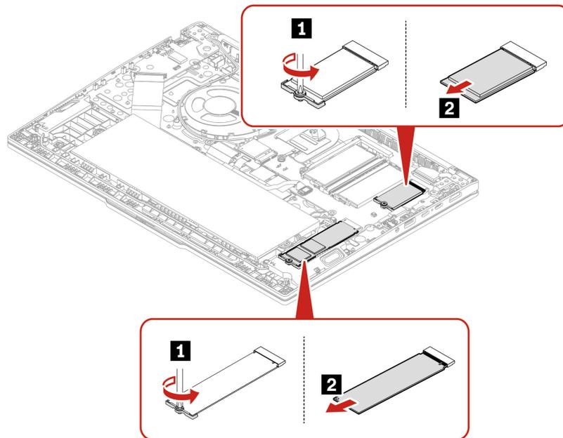
Step 2. Install the M.2 solid-state drive and its bracket as shown below. Fasten the captive screw to secure the M.2 solid-state drive.
