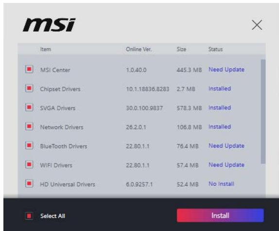
5. Check the **Select All** checkbox in the lower-left corner and click **Install** to install MSI Center and drivers. The installation progress will be shown at the bottom.
