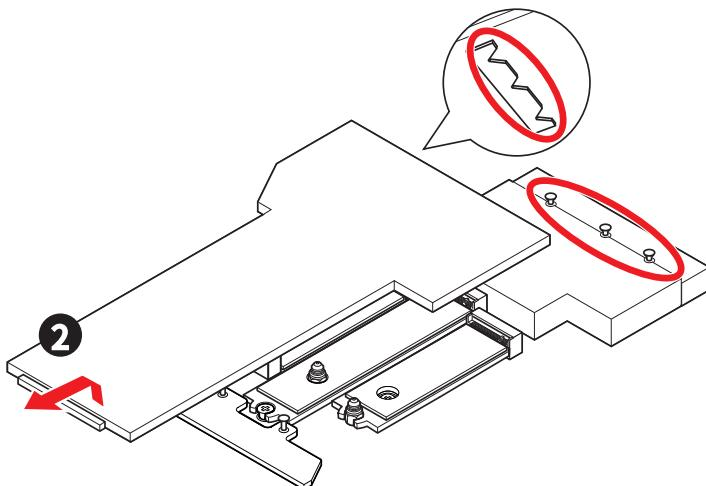
3. Remove the protective film from the M.2 thermal pads on the M.2 plate.
