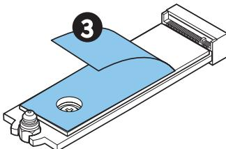
4. If you install 2260 or 22110 SSD, please exchange **EZ M.2 Clip II** and the **plate screw**. Use the included **EZ M.2 Clip II Remover** to install EZ M.2 Clip II in the slot. Skip this step if you install 2280 SSD.
