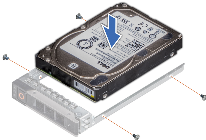
Figure 62. Installing a drive into the drive carrier
