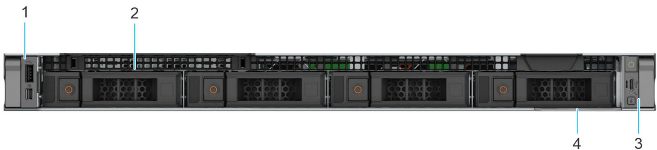
Figure 6. Front view of 4 x 3.5 inch -drive system with rear I/O
