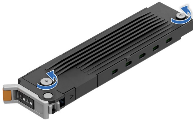
Figure 167. Loosen the top cover captive screws
