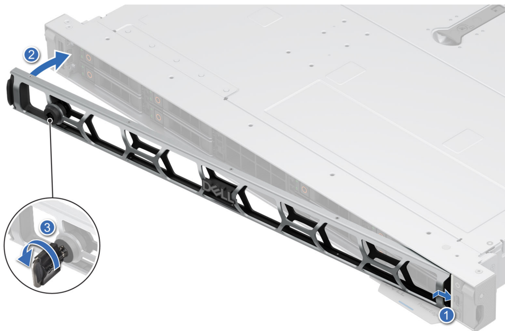
Figure 37. Installing the front bezel
