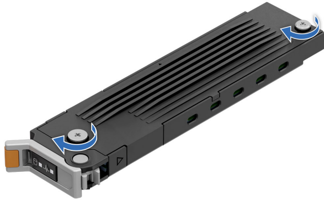
Figure 172. Tighten the top cover captive screws
