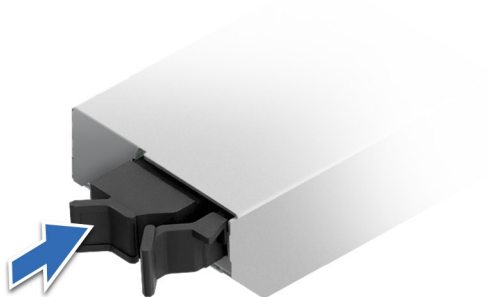
Figure 187. Installing the BOSS-N1 DC-MHS card carrier blank
