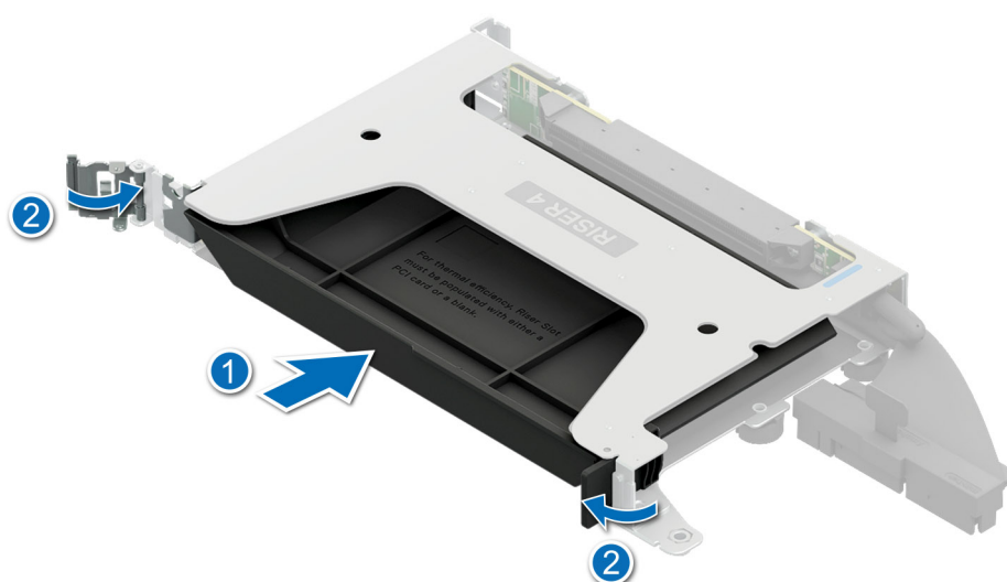
Figure 168. Installation du cache PCIe
