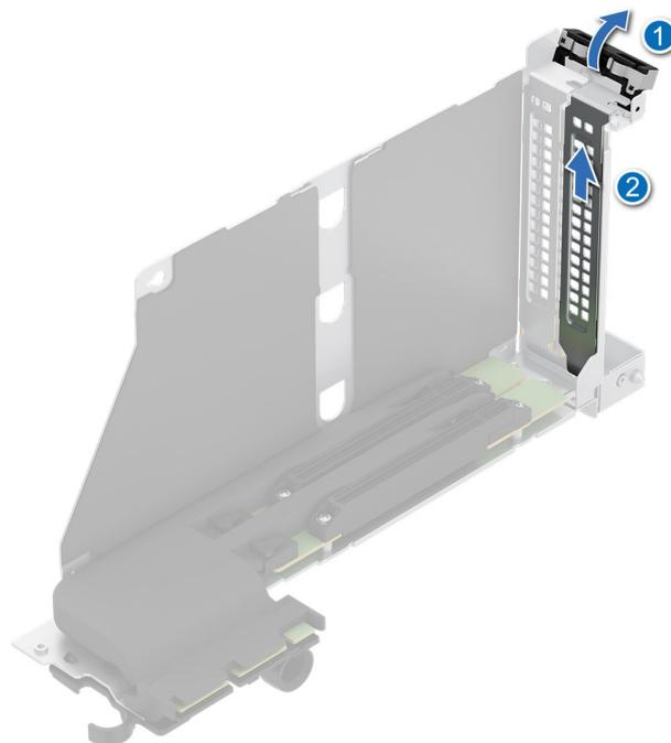
**Figure 174. Removing the filler bracket**
