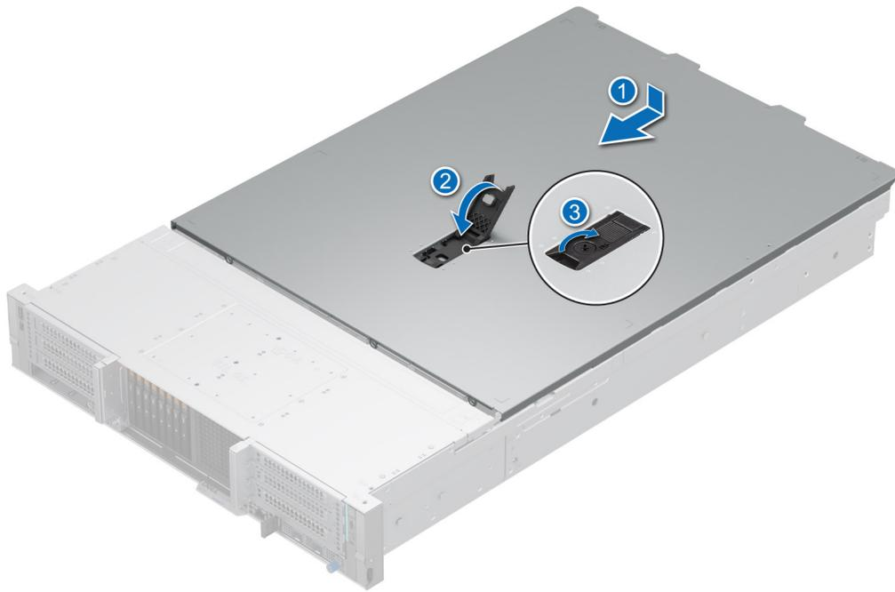
**Figure 35. Installing the system cover**
