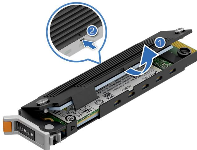
**Figure 188. Removing the top cover**
