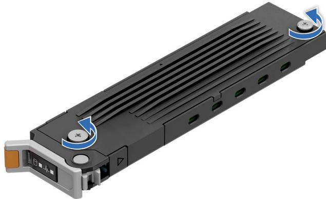
**Figure 187. Loosen the top cover captive screws**
