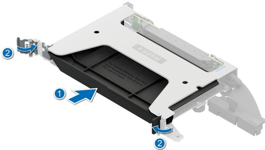
Figure 168. Installing the PCIe blank
