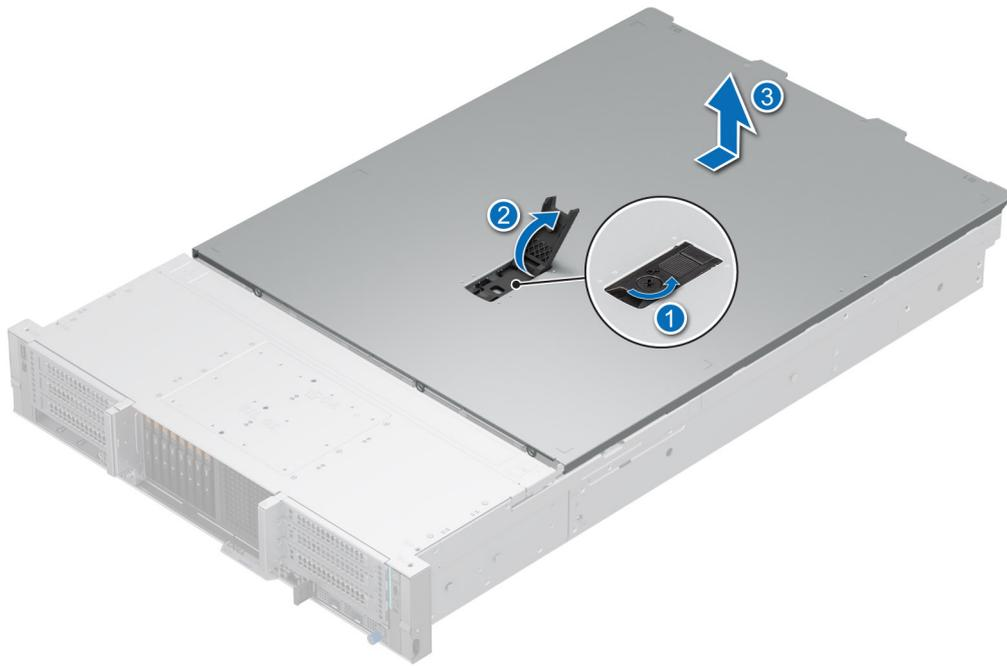
**Figure 34. Removing the system cover**
