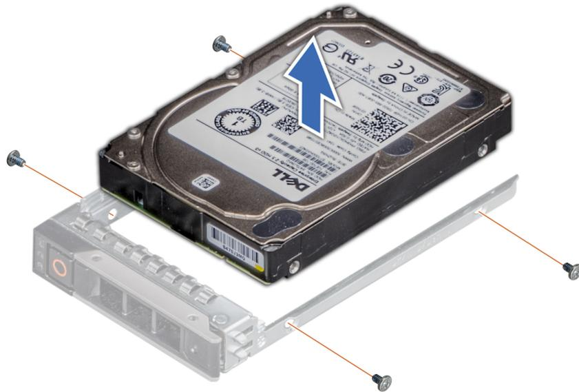
**Figure 63. Removing the 3.5-inch drive from the drive carrier**
