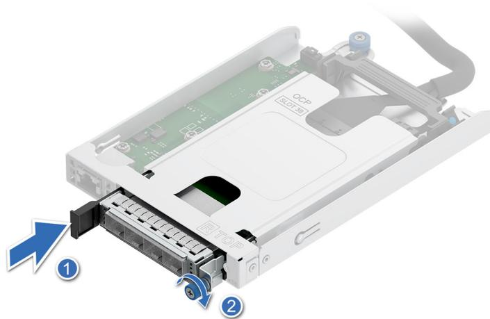
**Figure 239. Installing the OCP NIC tray into riser**
