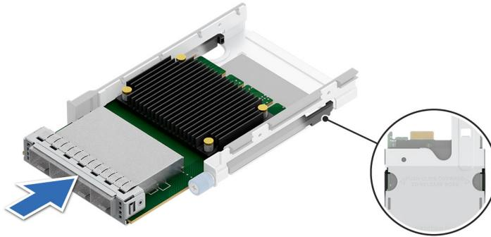
**Figure 237. Installing an OCP NIC card into OCP tray**
