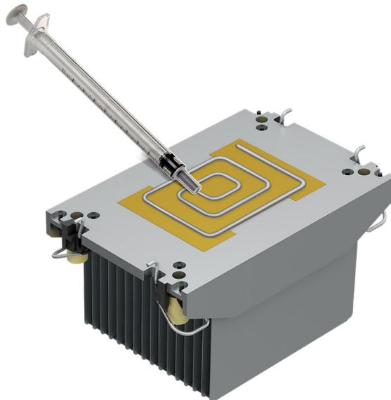
**Figure 119. Applying thermal grease**
