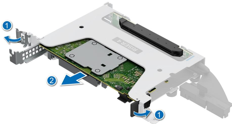
**Figure 166. Removing the expansion card from the riser 4**
