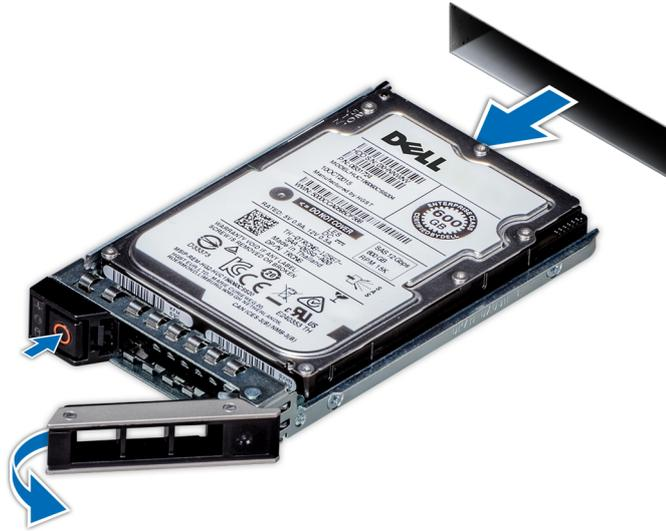
Figure 62. Removing a 3.5-inch drive carrier
