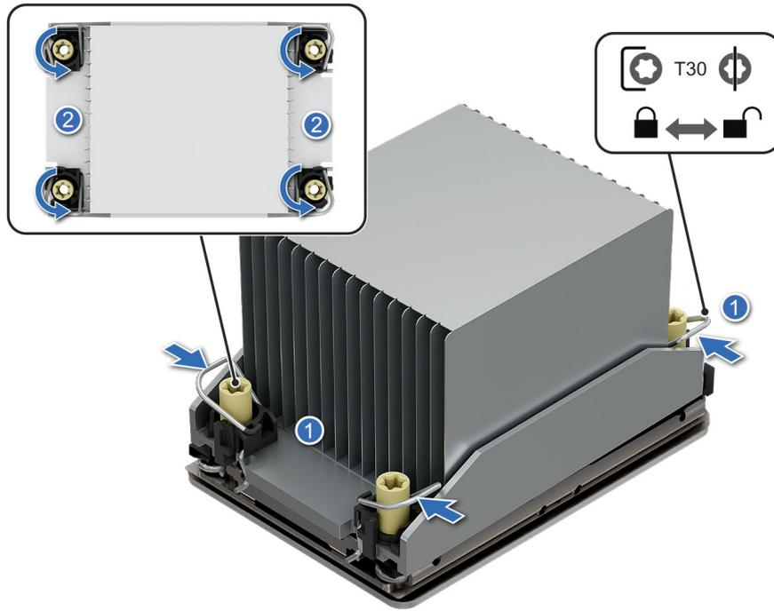
**Figure 113. Removing the processor heat sink module**
