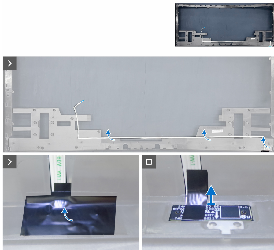
Figure 35. Retrait du câble LED
