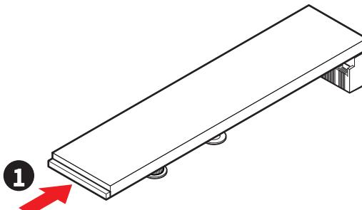
2. Slightly lift up the end part of Screwless M.2 Shield Frozr heatsink and move it forward to uninstall the heatsink.
