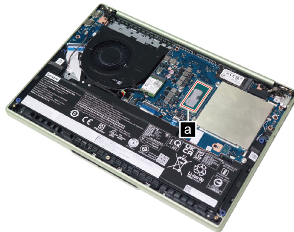
Figure 17. Areas on the system board where thermal interface materials are applied (for Intel models)
