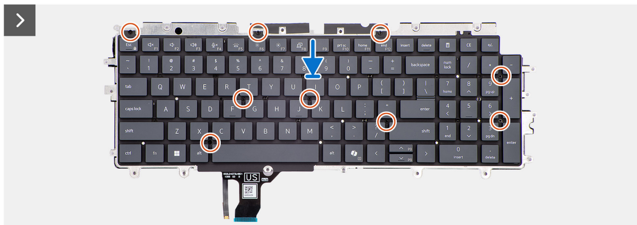
Figure 85. Installation du clavier
