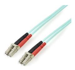
The A50FBLCLC2, 2-meter (6.6ft), 10 Gigabit, Aqua Multimode 50/125 Duplex LSZH Fiber Patch Cable is terminated at both ends with LC (male) connectors and is composed of 50/125 micron OM3 aqua fiber to deliver reliable data transfers at blinding speeds making it perfect for fiber cable runs between multiple backbone switches, hubs and routers as well as higher end networking equipment.
