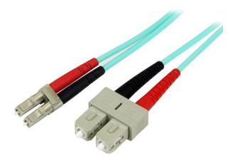
The A50FBLCSC2 2-meter (6.6ft), 10 Gigabit, Aqua Multimode 50/125 Duplex LSZH Fiber Patch Cable is terminated with one LC (male) connector and one SC (male) connector and is composed of 50/125 micron OM3 aqua fiber to deliver reliable data transfers at blinding speeds making it perfect for fiber cable runs between multiple backbone switches, hubs and routers as well as higher end networking equipment.
