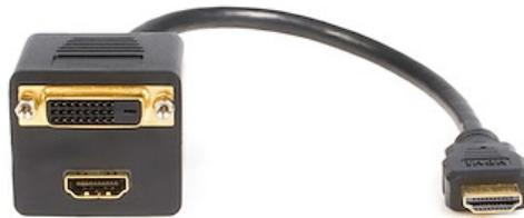
The HDMISPL1DH 1-foot HDMI to HDMI + DVI-D Splitter Cable splits a Computer or Satellite Receiver's HDMI output signal into one DVI and one HDMI output, allowing you to view content on one DVI display and one HDMI-capable display simultaneously.
