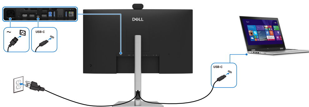
Figure 39. Branchement du câble USB-C
