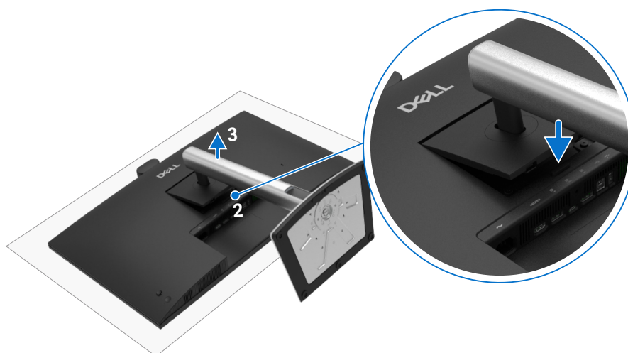
Figure 60. Removing the monitor stand
