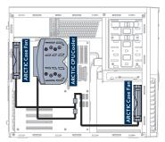
The PST ensures all PWM-controlled devices run at optimized speed (and hence lower noise level) based on actual CPU cooling demand.
