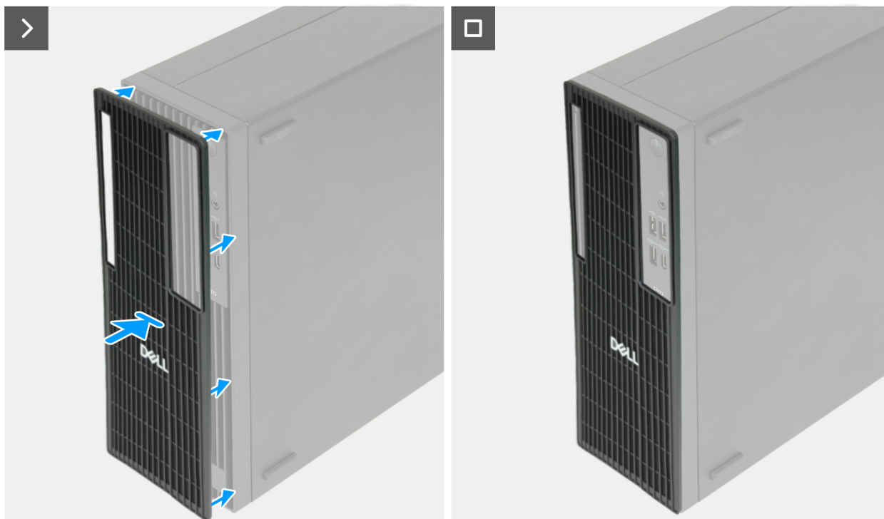
Figure 15. Installation du filtre anti-poussières
