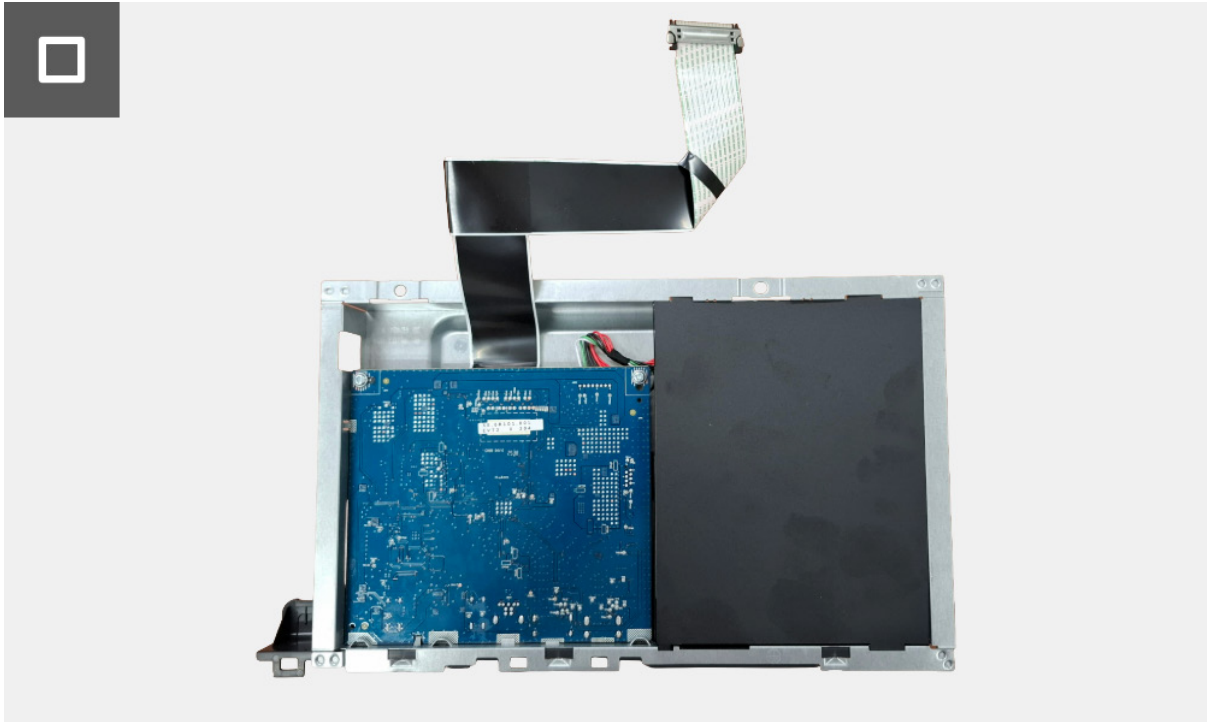
Figure 11. Removing the metal shield
