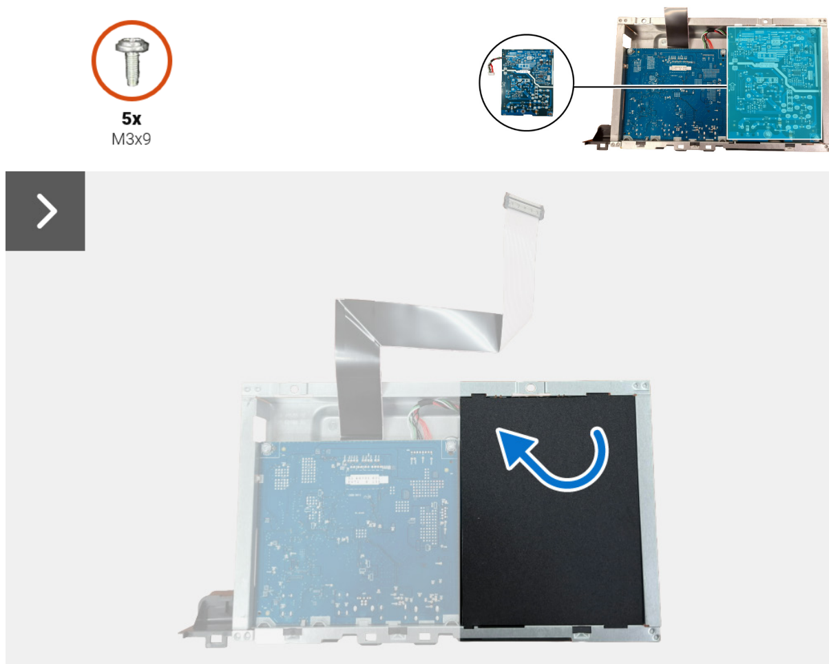
Figure 16. Removing the power board
