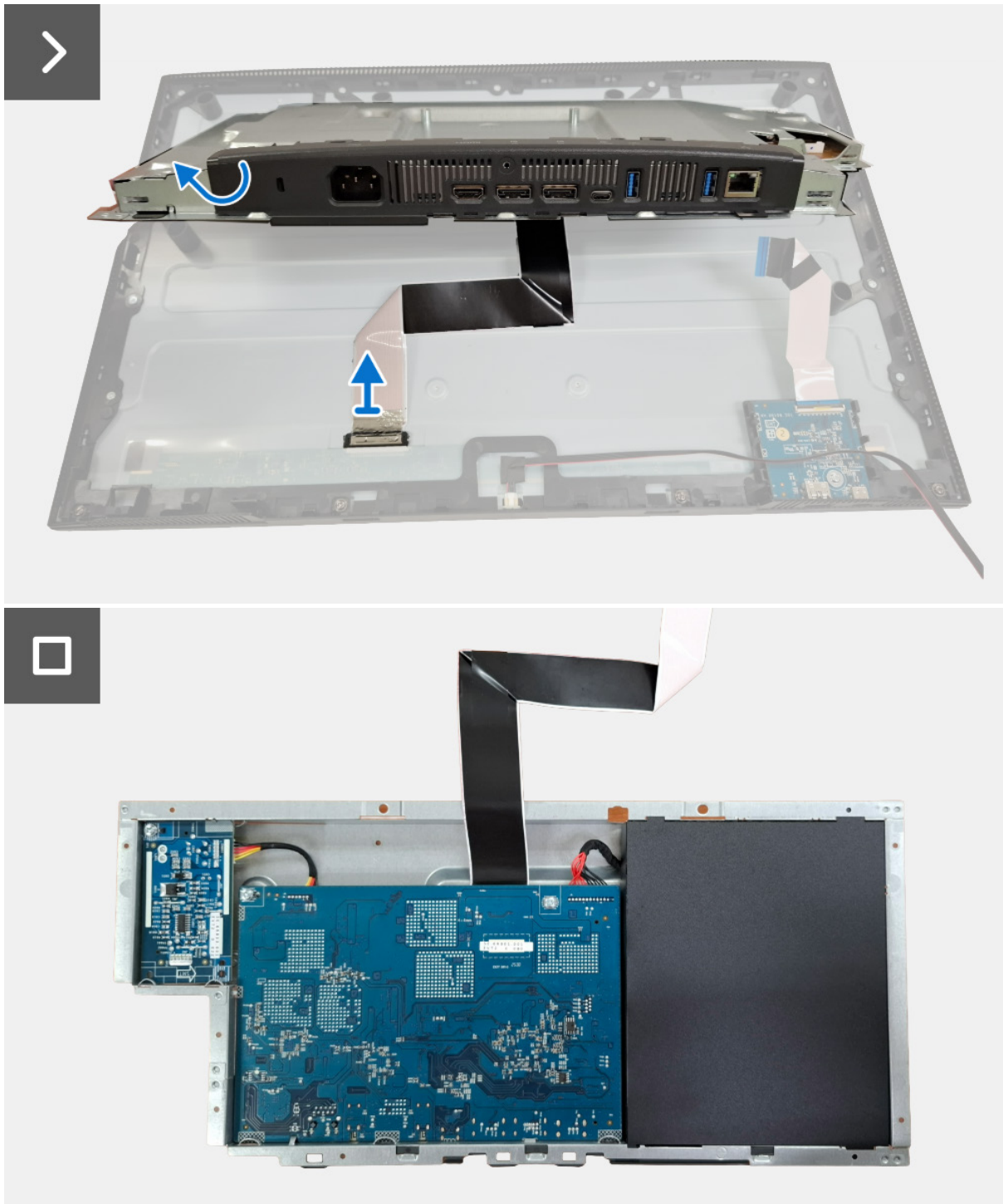
Figure 10. Removing the metal shield
