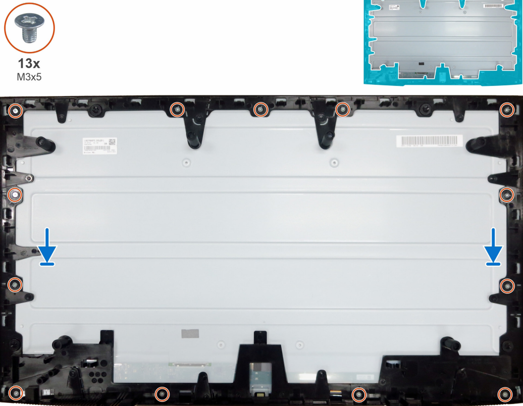
Figure 14. Installing the middle frame
