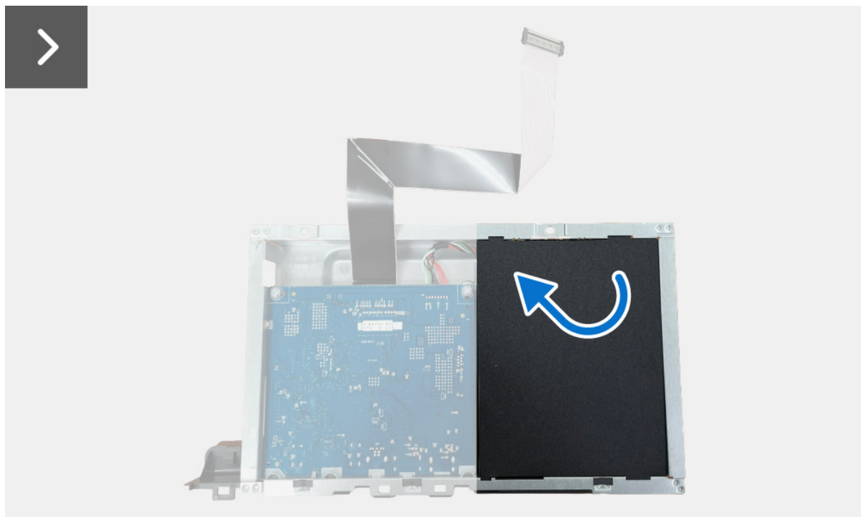
Figure 14. Removing the power board
