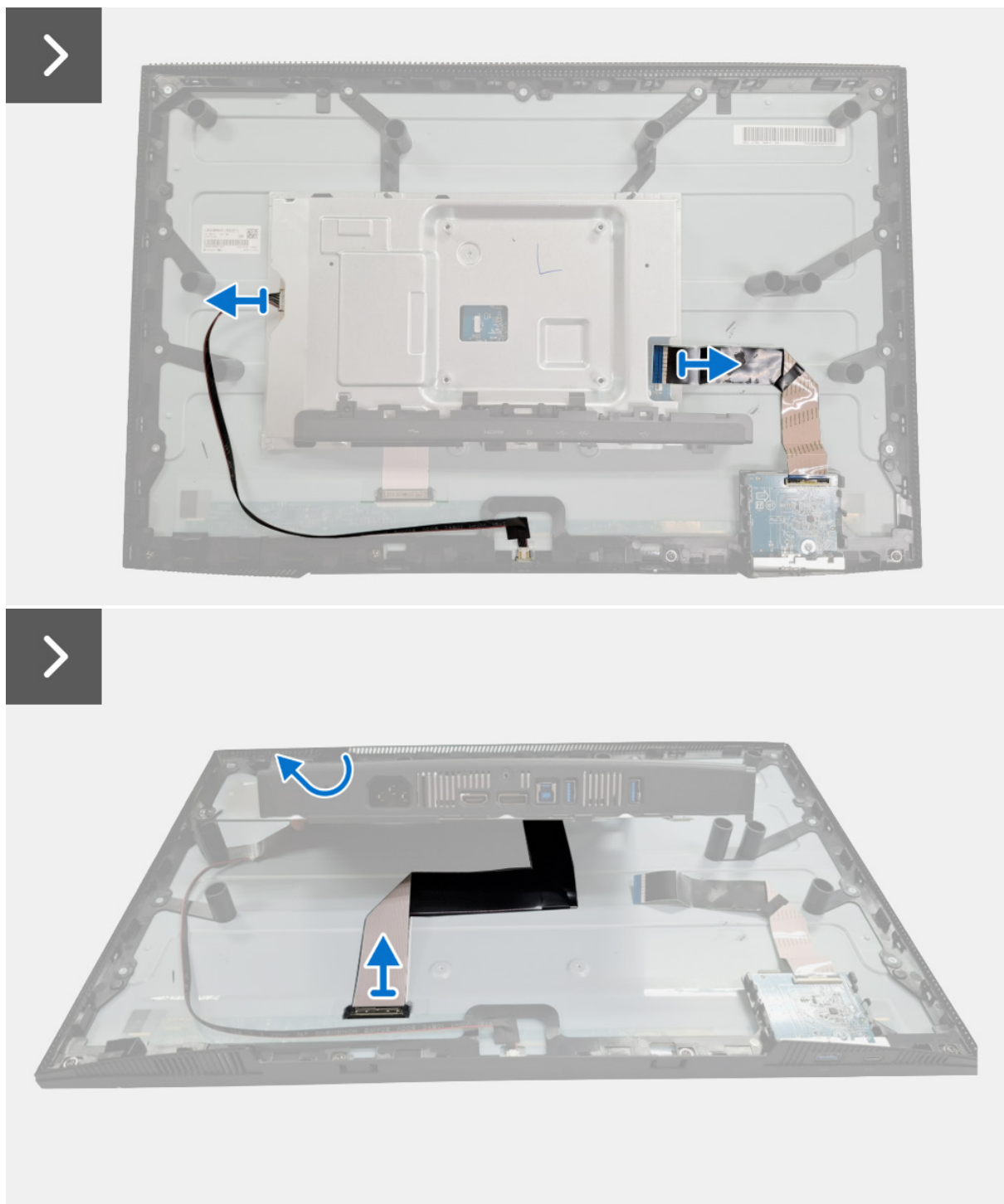
Figure 9. Removing the metal shield
