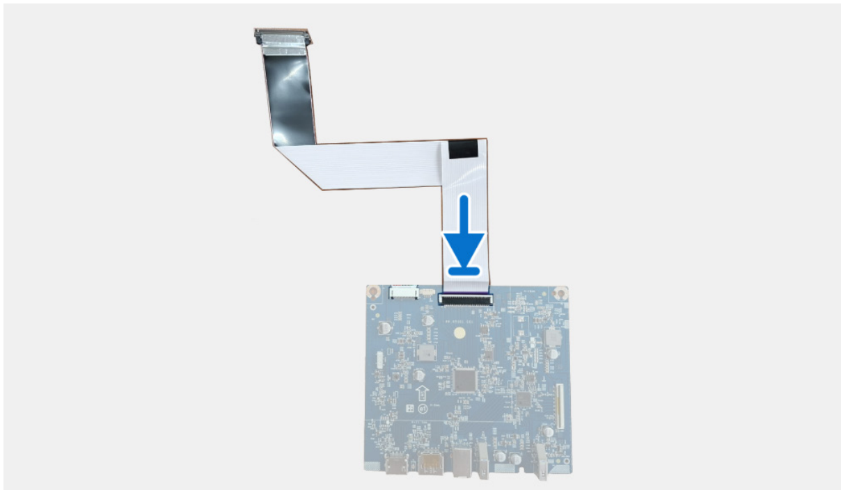
Figure 21. Installing the interface board
