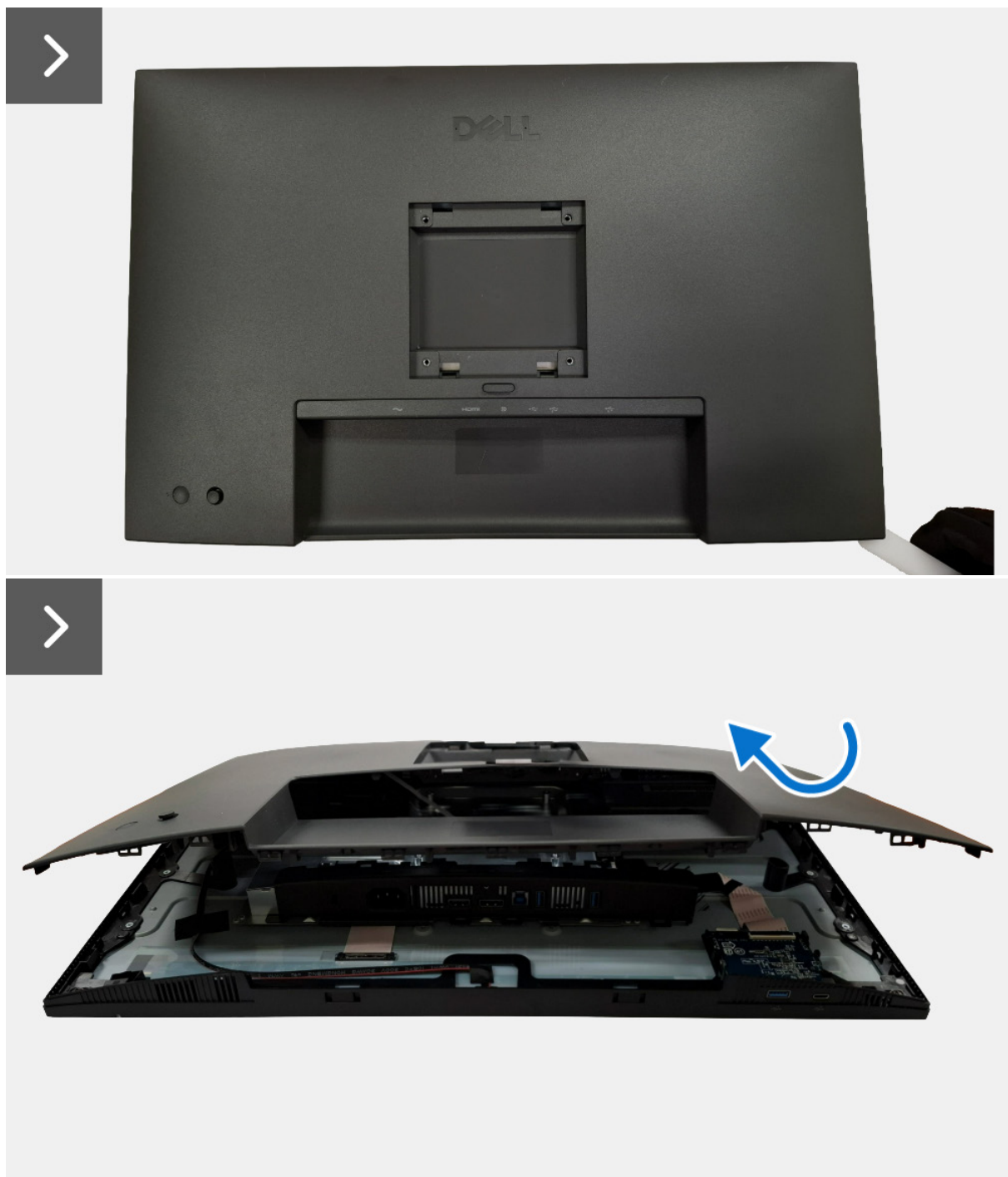
Figure 14. Removing the back cover
