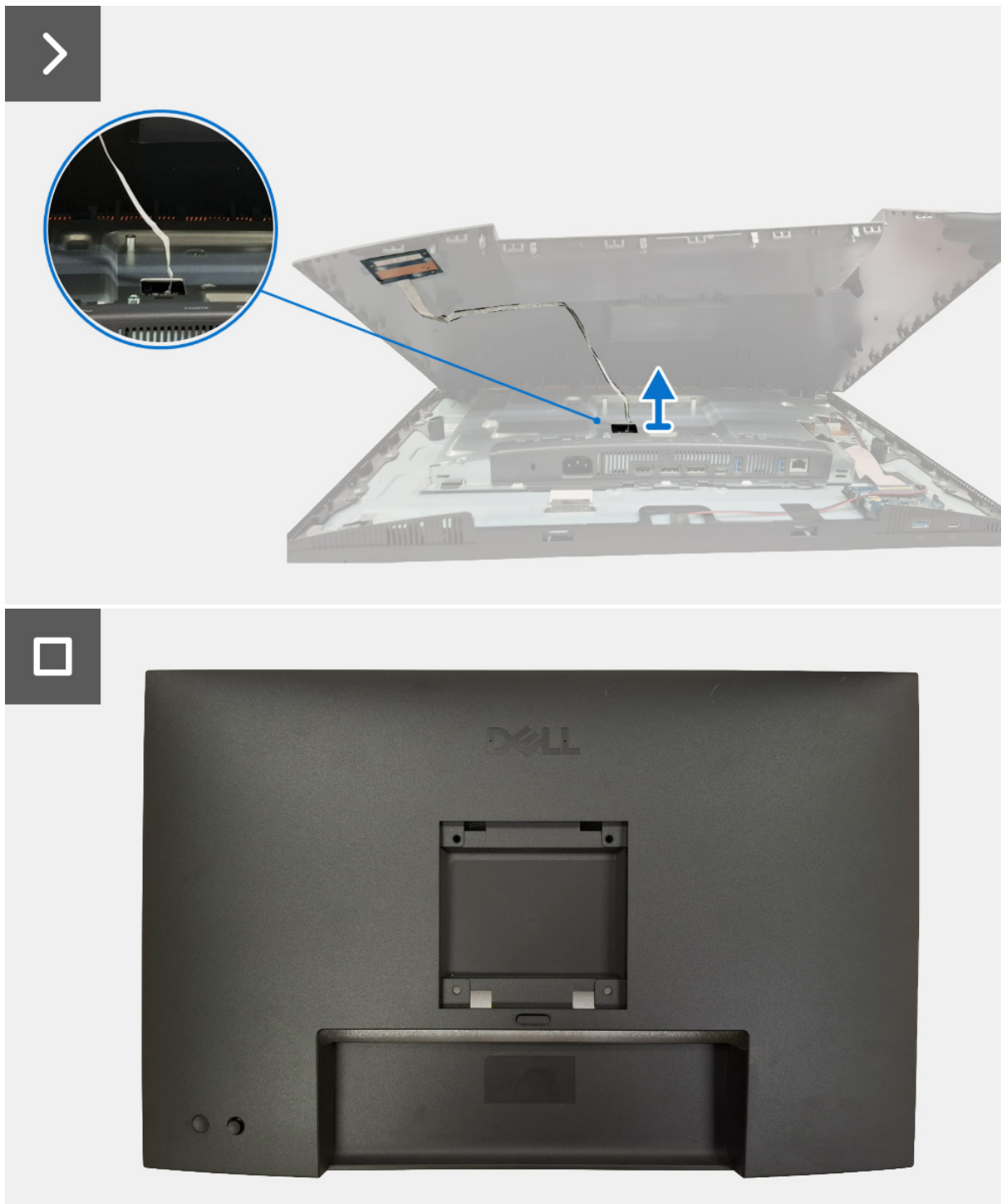
Figure 15. Removing the back cover
