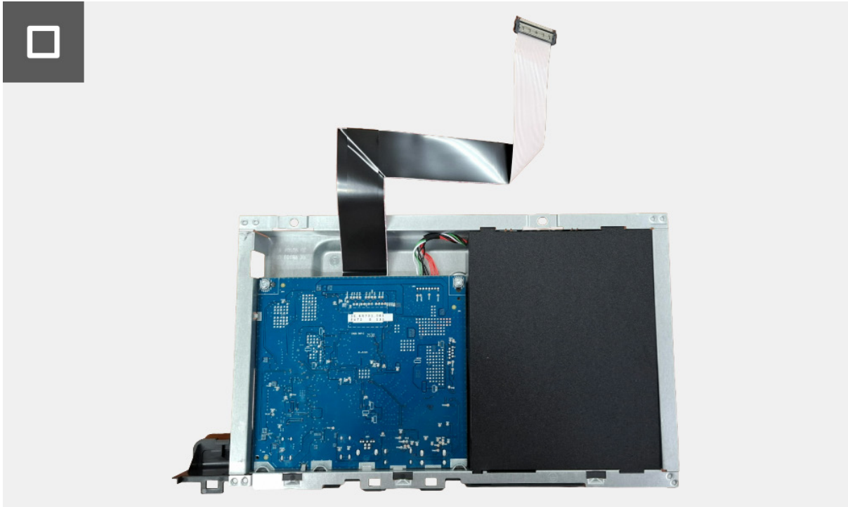
Figure 20. Removing the metal shield
