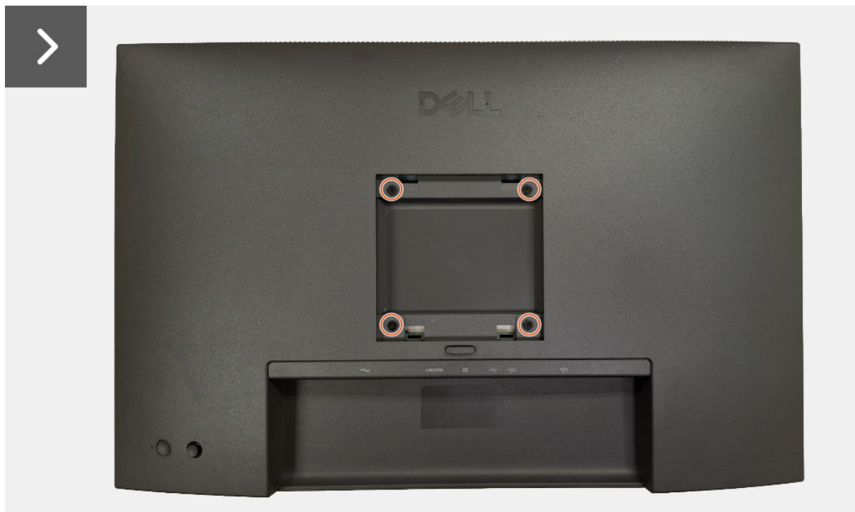
Figure 13. Removing the back cover
