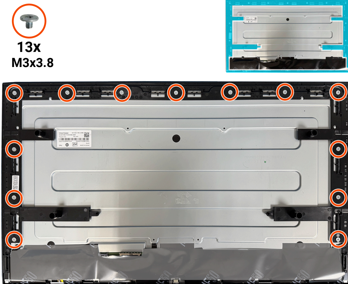
Figure 18. Installer le cadre central
