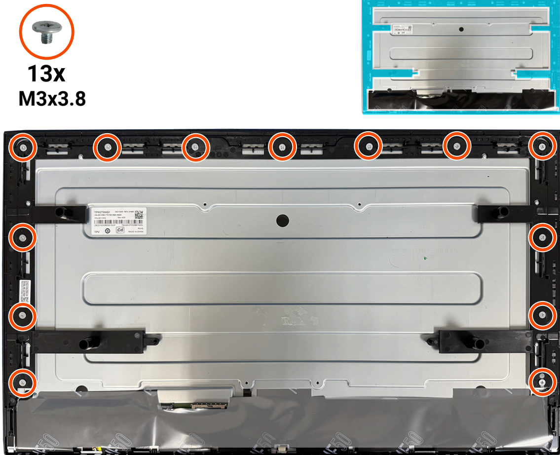
Figure 29. Installing the middle frame
