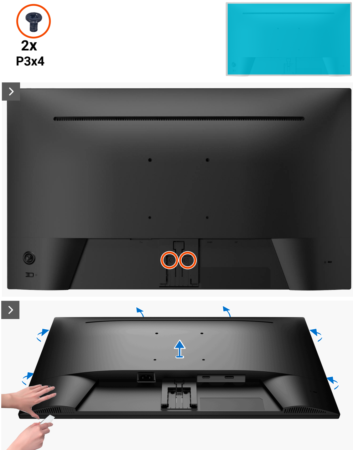
Figure 14. Removing the back cover
