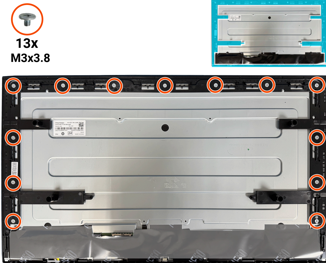
Figure 28. Removing the middle frame
