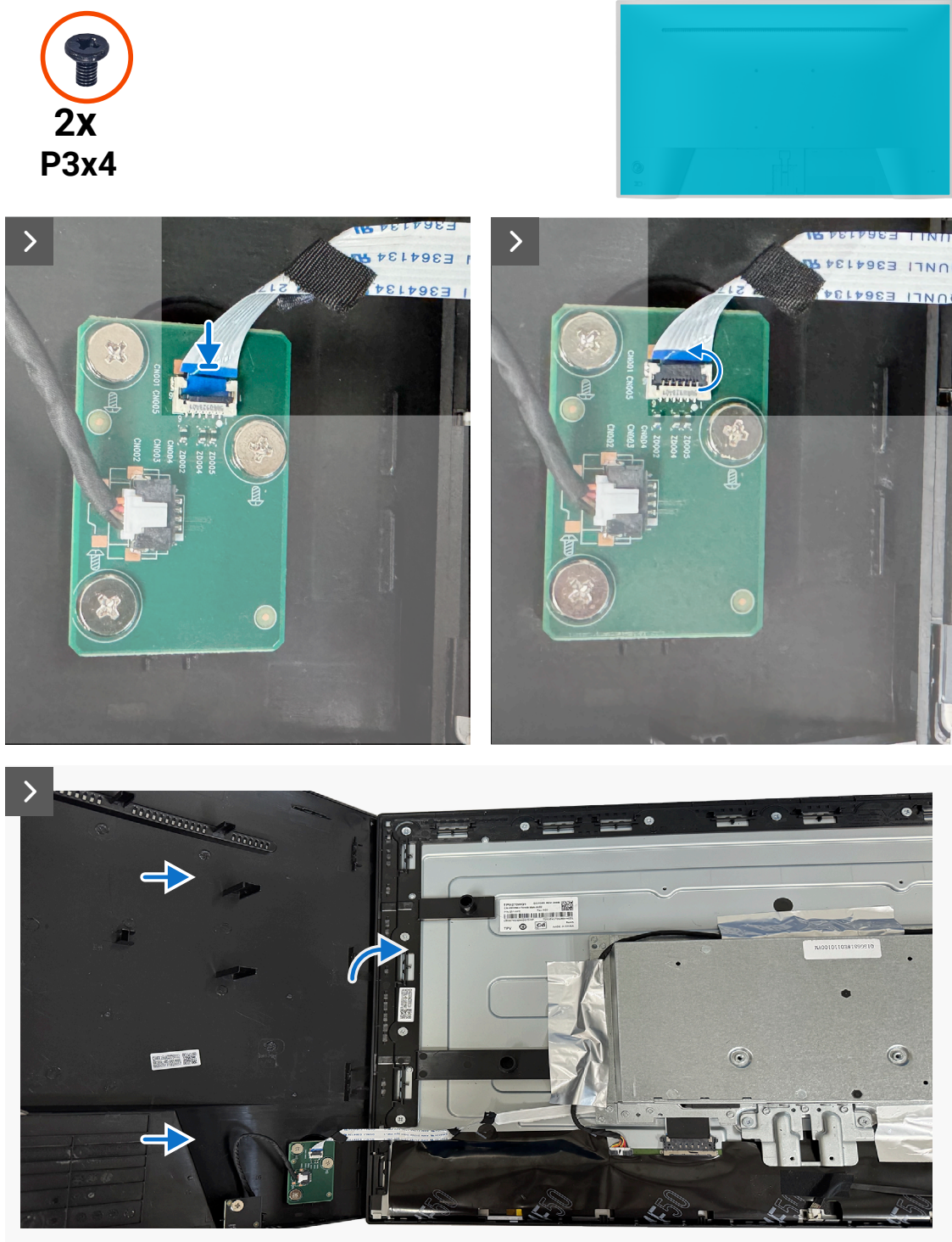
Figure 16. Installing the back cover
