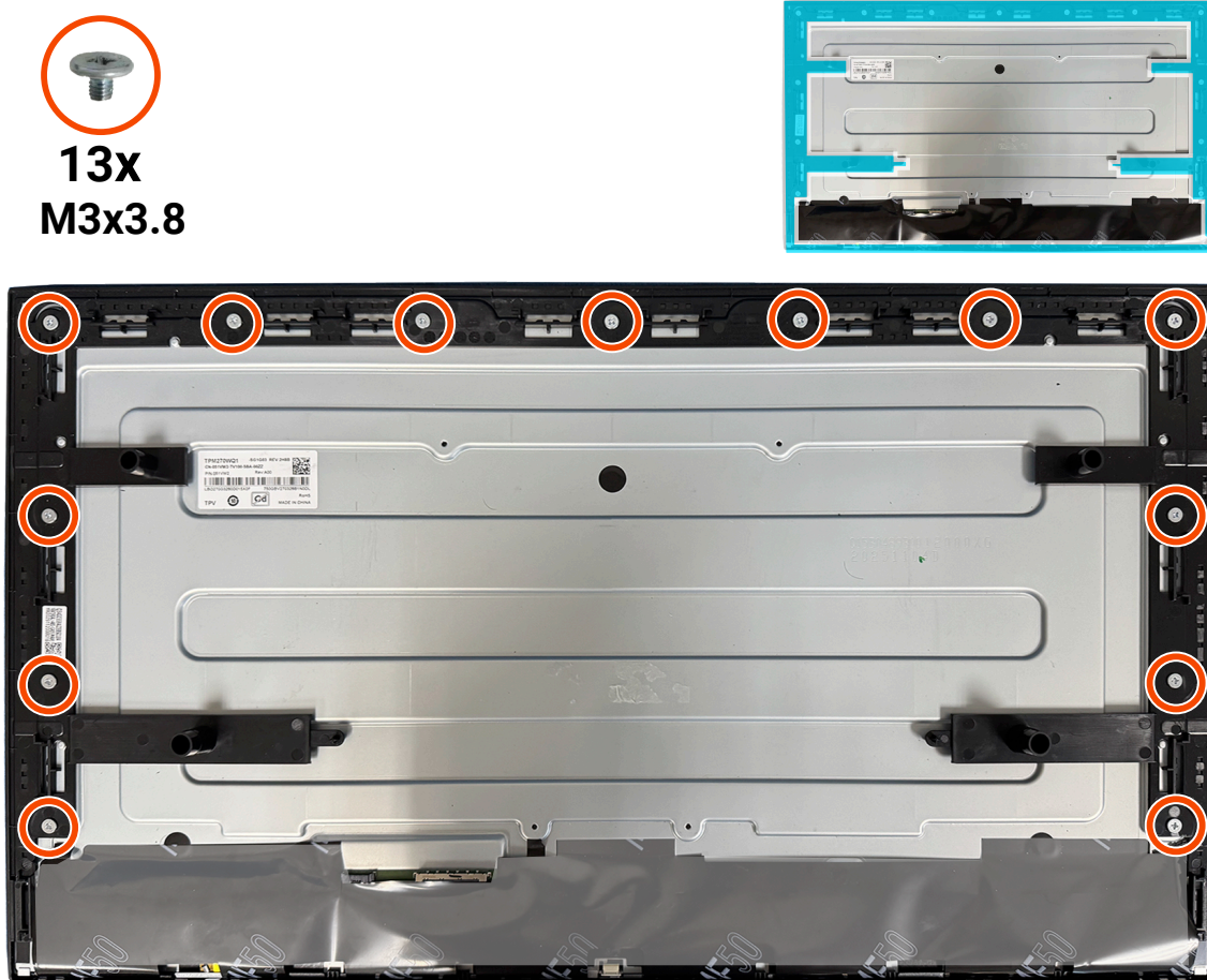
Figure 17. Removing the middle frame
