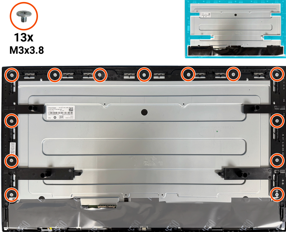
Figure 18. Installing the middle frame
