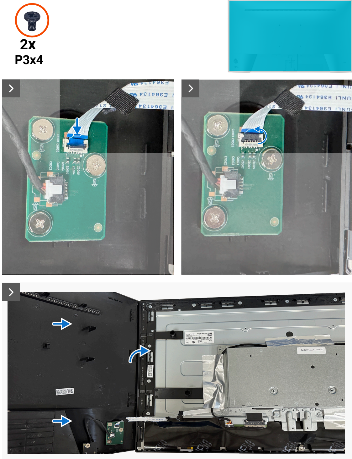
Figure 5. Installing the back cover
