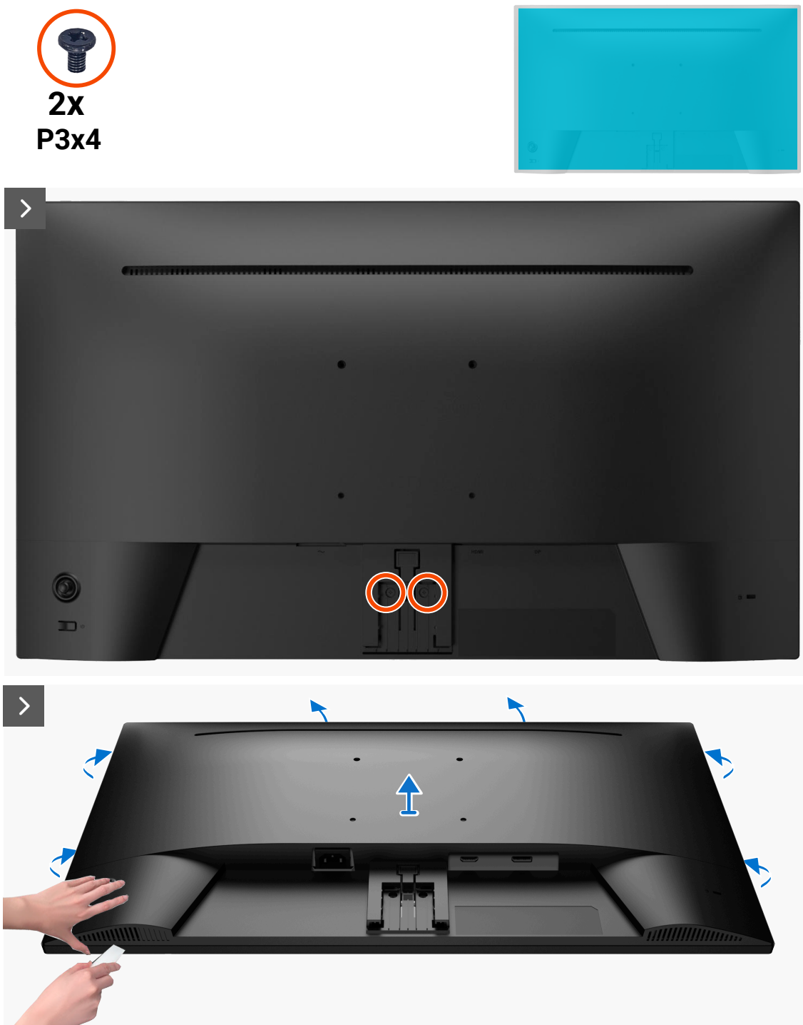
Figure 3. Removing the back cover
