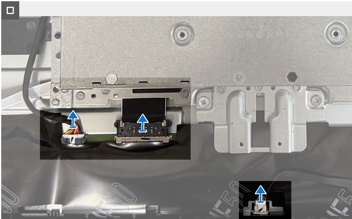
Figure 10. Removing the metal shield
