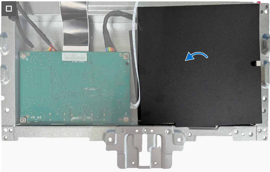
Figure 16. Installing the system board and power board
