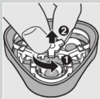
**2** Press the release button (1) and remove the shaving unit (2).
