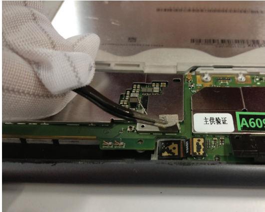
Figure 5. Removal steps of front camera
