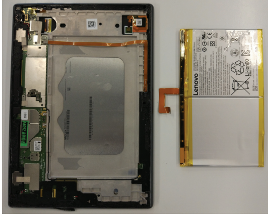
Figure 2. Removal steps of battery (continued)
