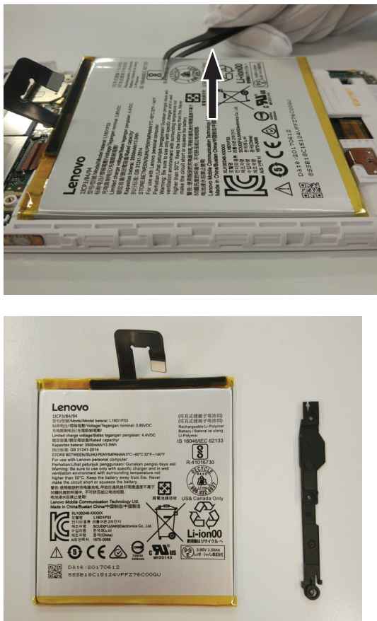
Figure 2. Removal steps of battery (continued)
