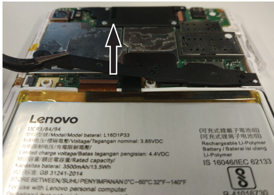
Figure 2. Removal steps of battery (continued)
