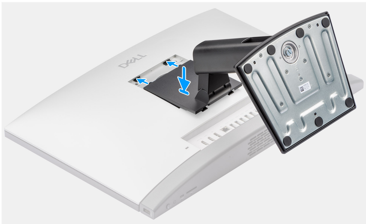
Figure 20. Installing the Fixed Stand
