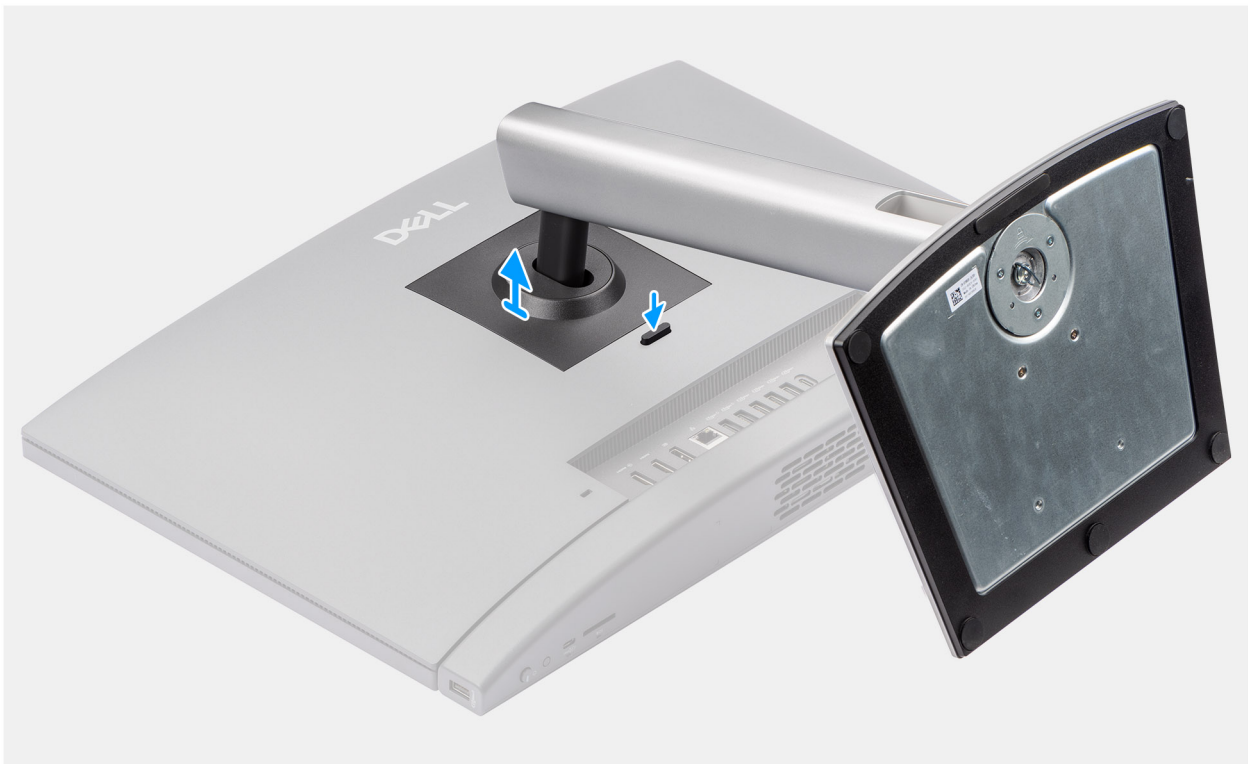
Figure 14. Removing the Height Adjustable Stand (HAS)
