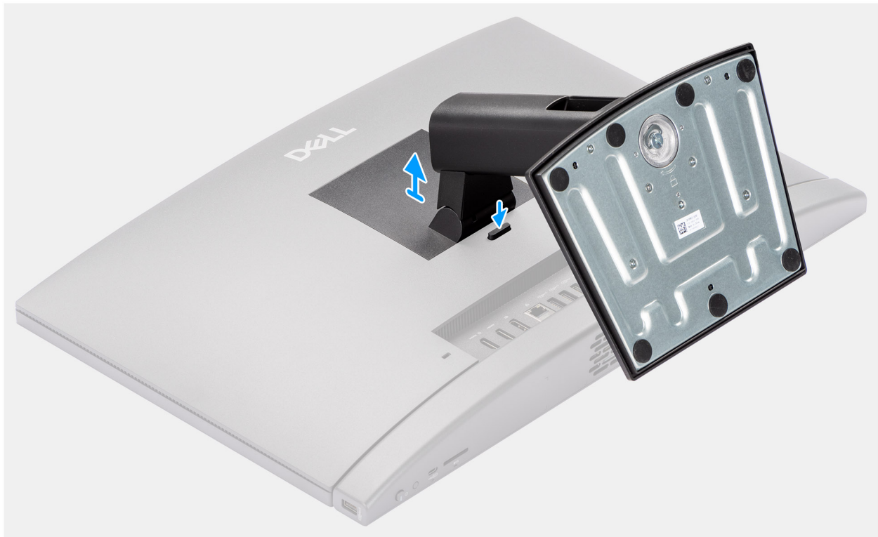
Figure 15. Removing the Fixed Stand
