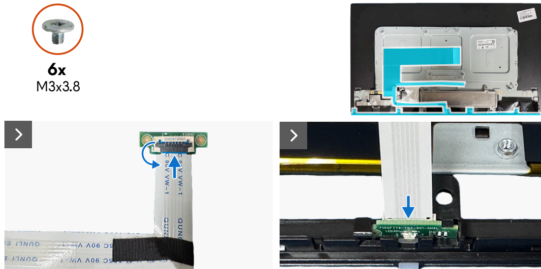
Figure 17. Installer la carte LED
