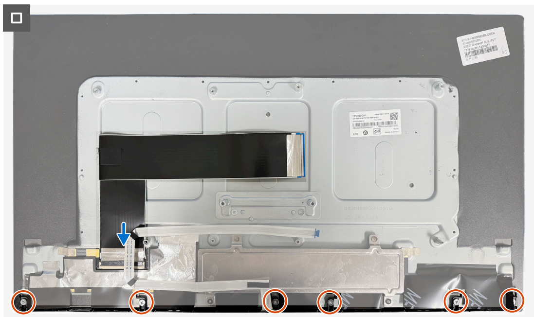
Figure 18. Installer la carte LED
