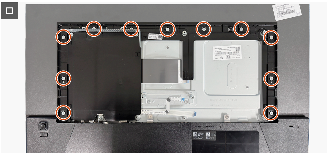
Figure 22. Installer le cadre central
