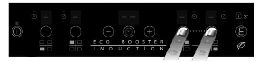
To change the power level, press the -/+ buttons (from 1 to a maximum of 9 or P). To deactivate the Flexi cook function, press simultaneously the 2 selecting buttons of the zones. To switch off the zones instantly, hold one of the zone selection button for 3 seconds.
