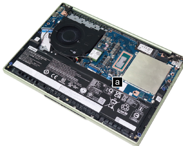
Figure 16. Area on the system board where thermal interface materials are applied (for Intel models)
