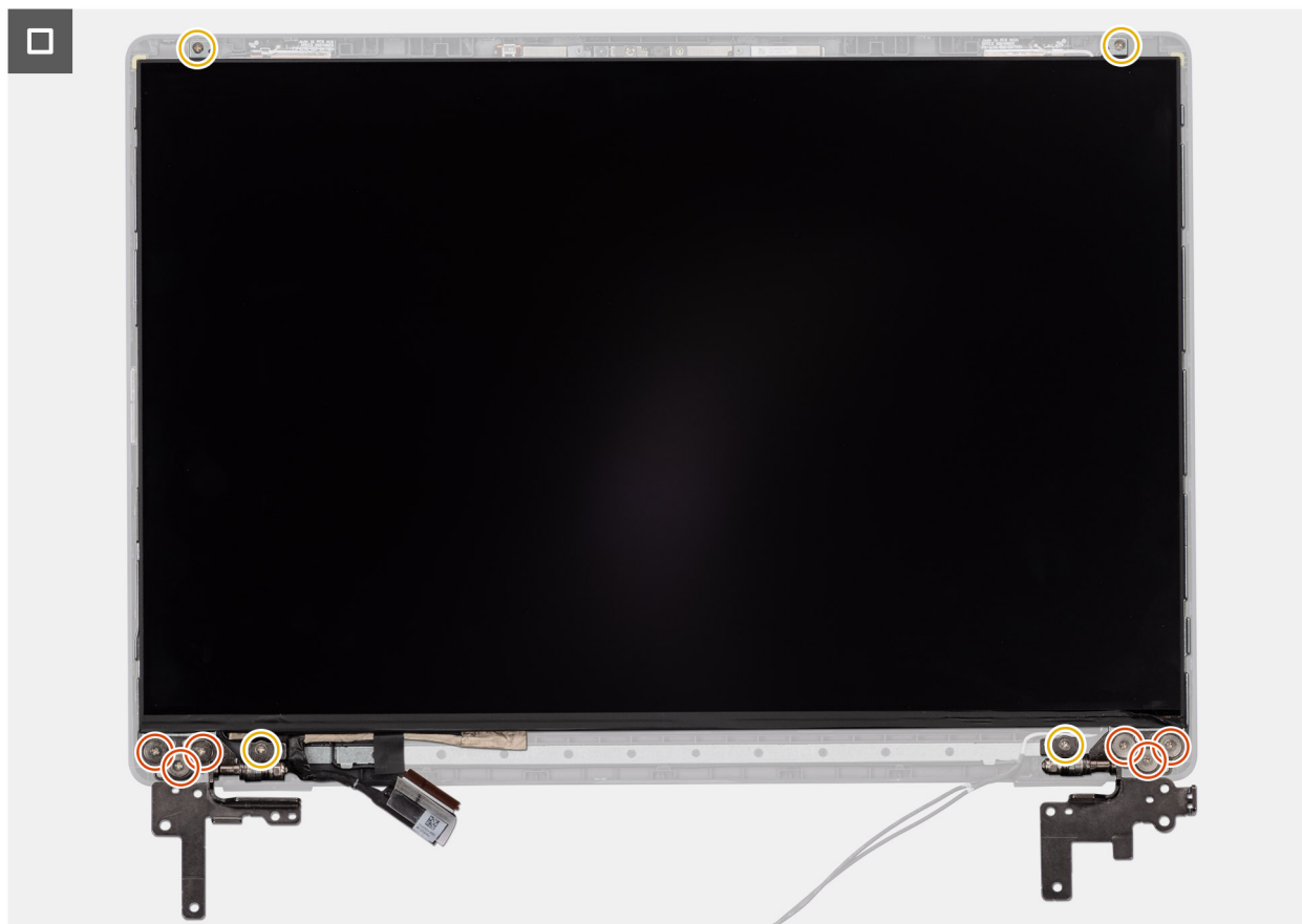
Figure 112. Installing the display-panel assembly
