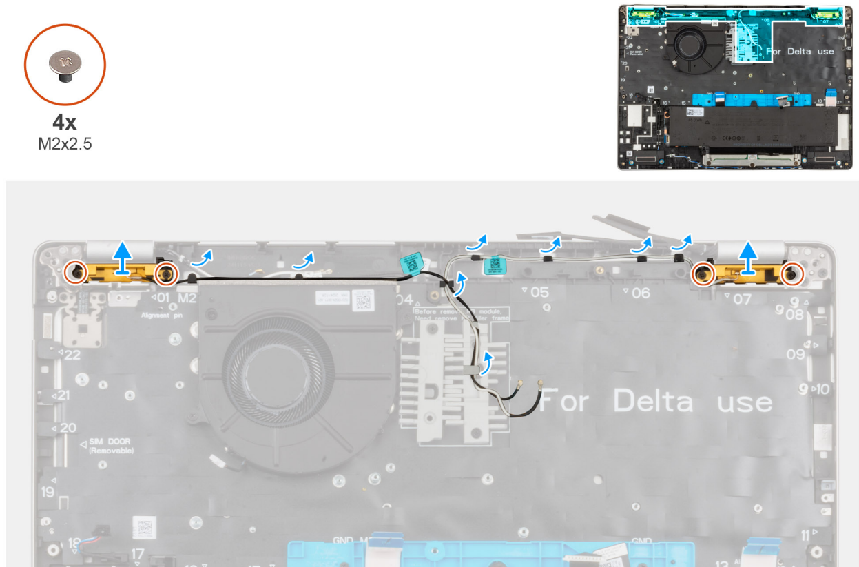
Figure 78. Removing the WLAN antenna module
