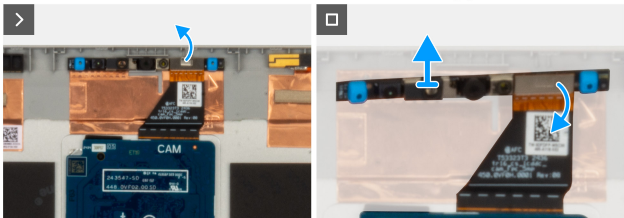
Figure 74. Removing the camera module
