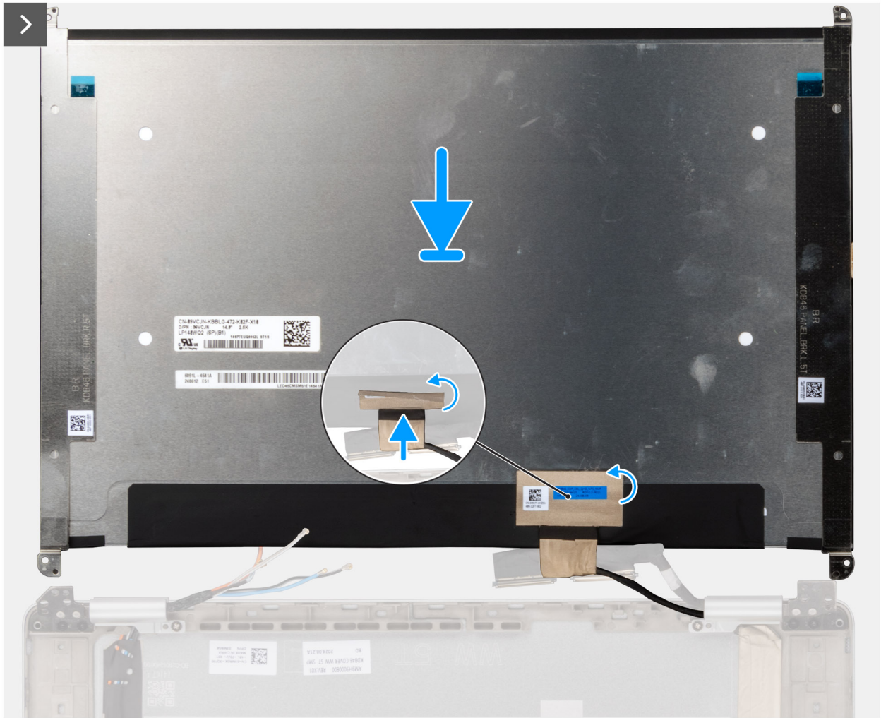
Figure 75. Installing the display panel
