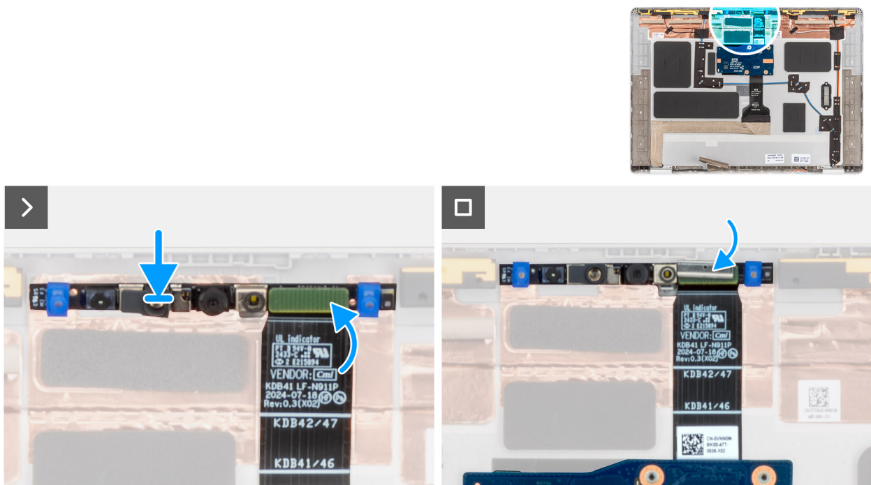
Figure 84. Installing the MIPI camera
