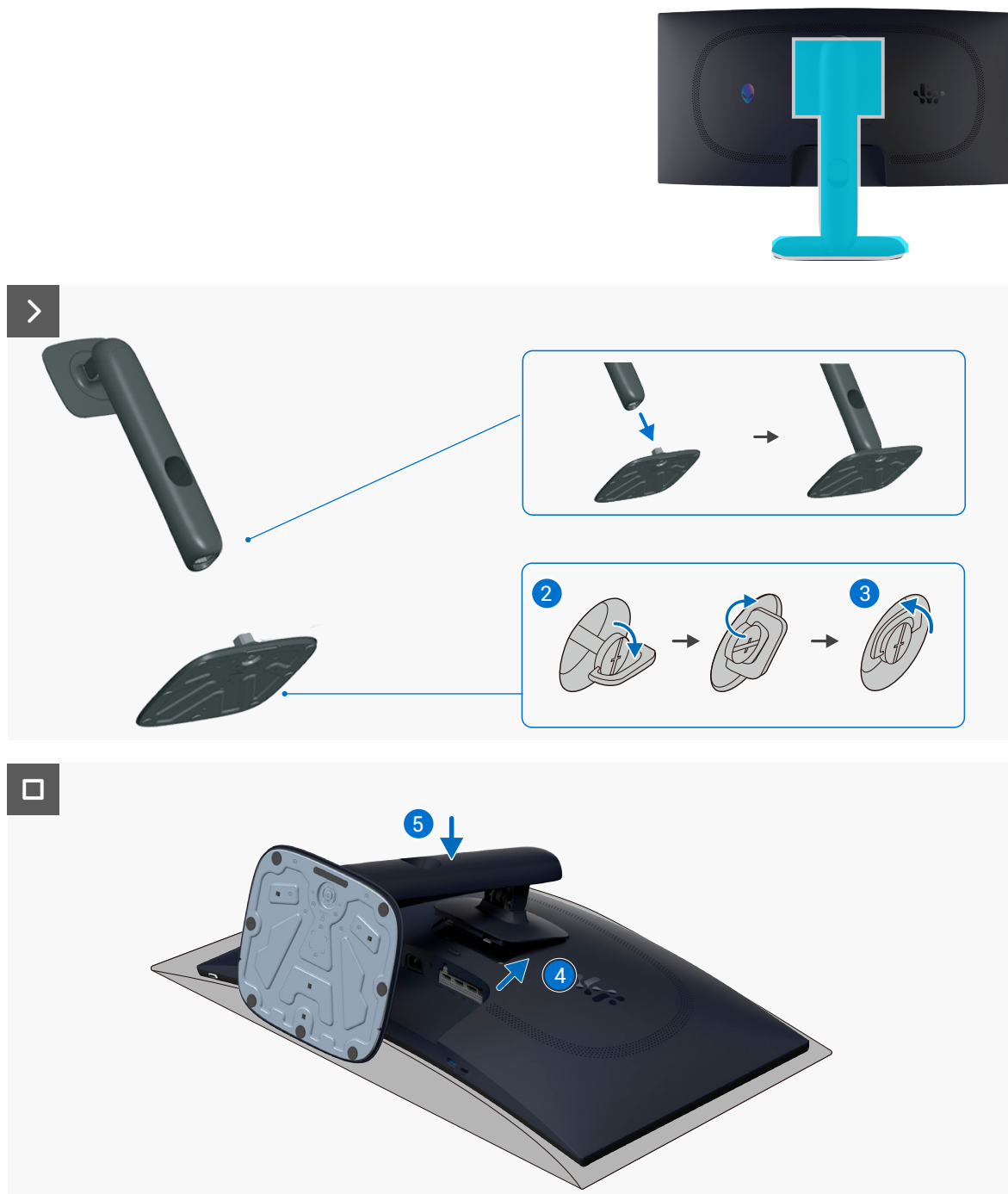
Figure 15. Installer le socle
