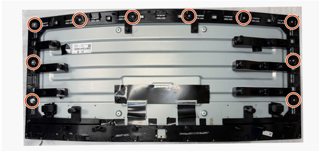
Figure 34. Installer le cadre central
