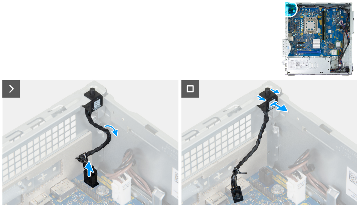
Figure 42. Removing the intrusion switch
