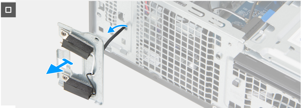
Figure 46. Removing the antenna modules
