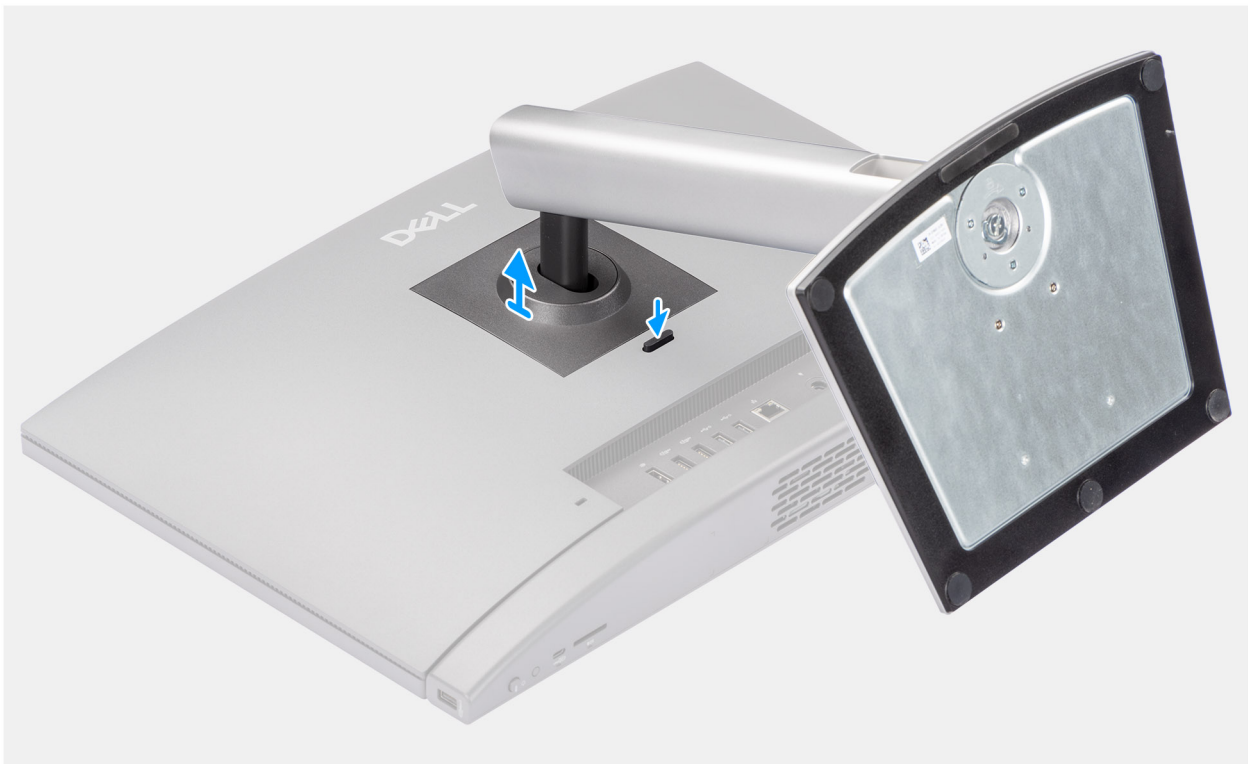
Figure 14. Removing the Height Adjustable Stand (HAS)
