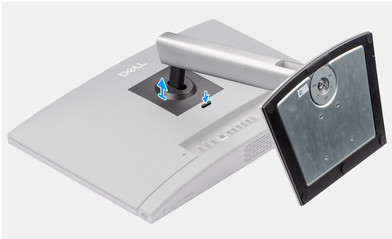
Figure 13. Removing the Height Adjustable Stand (HAS)
