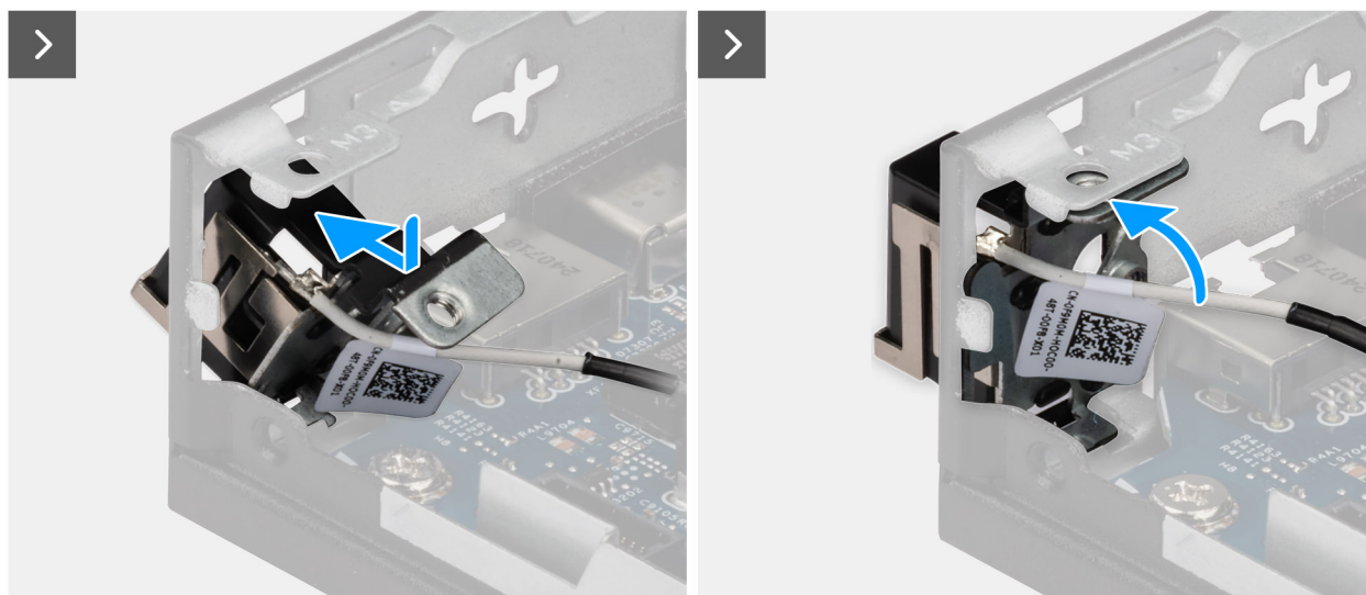
Figure 75. Installing the antenna module (white cable)
