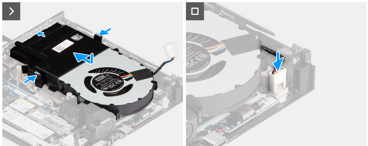
Figure 31. Installing the fan
