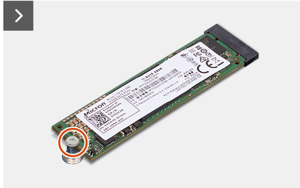
Figure 24. Removing the M.2 2280 solid state drive from slot 0
