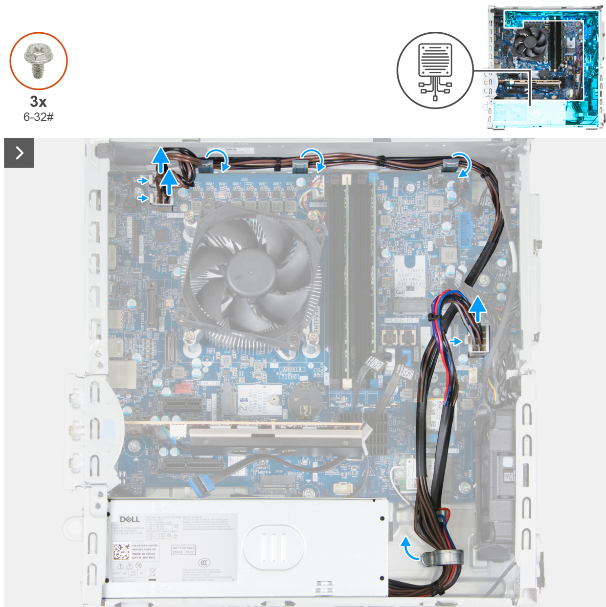
Figure 70. Installing the power-supply unit
