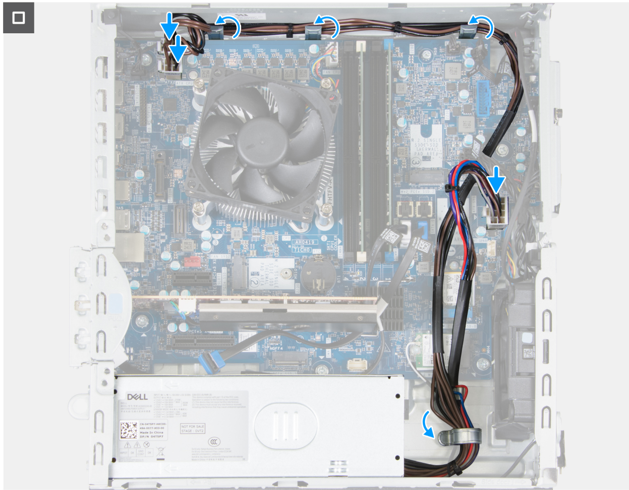
Figure 73. Installing the power-supply unit
