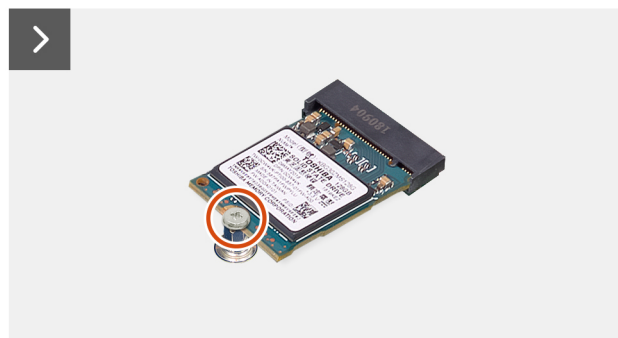
Figure 27. Removing the M.2 2230 solid state drive from slot 1
