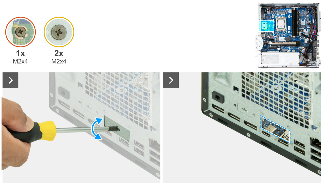
Figure 82. Installing the fiber-optic port module
