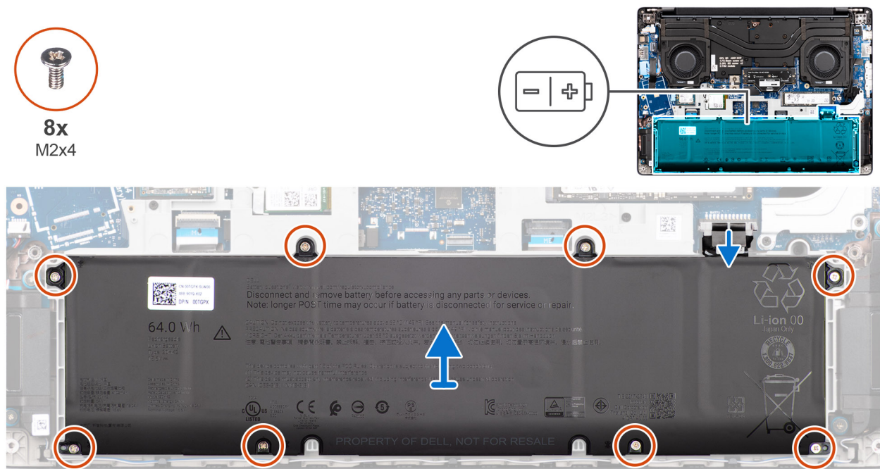
Figura 6. Removing the battery
