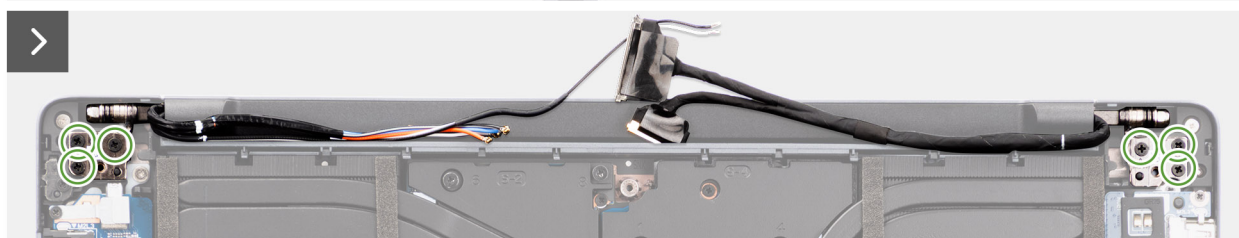
Figura 46. Installing the display assembly
