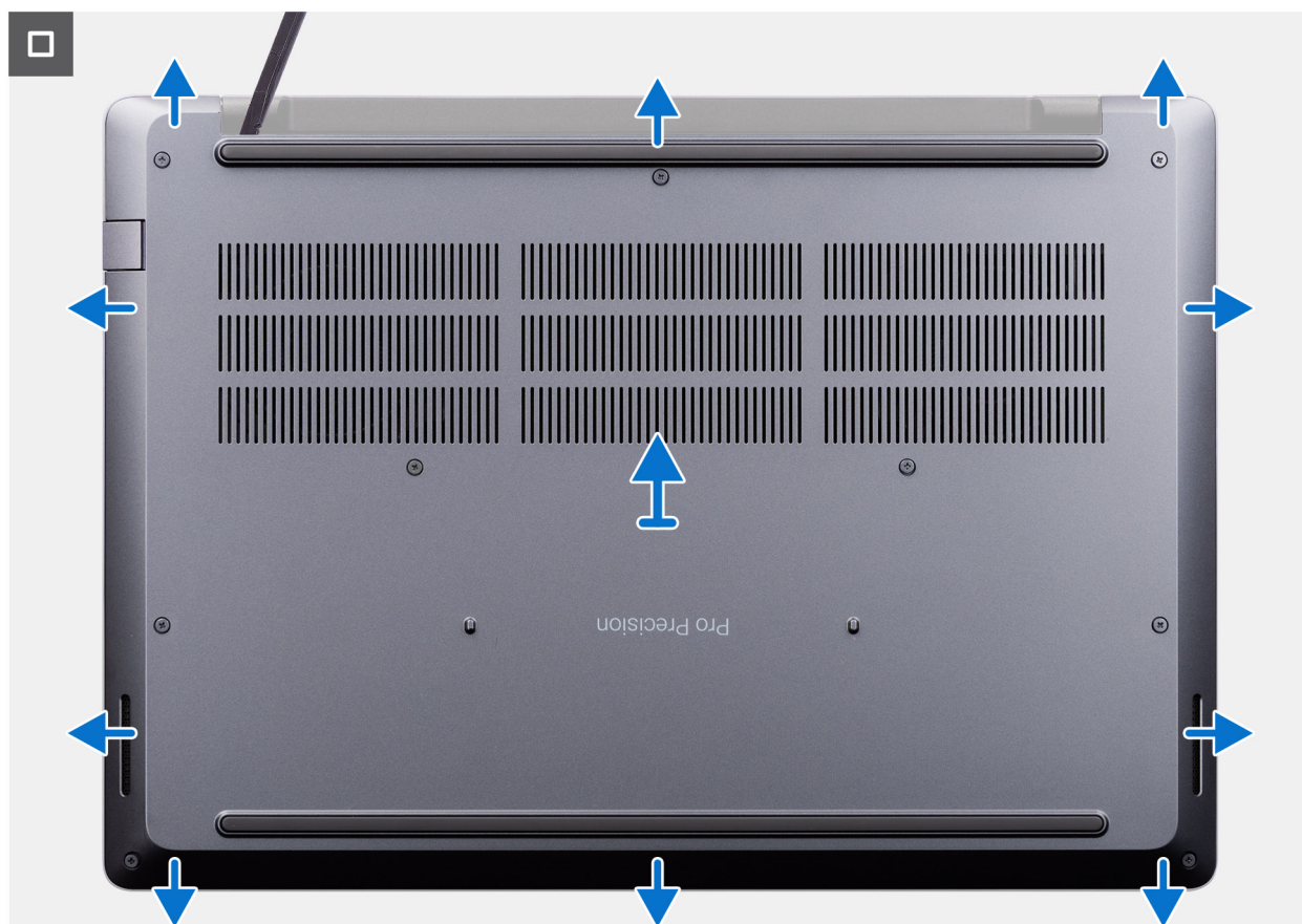
Figura 3. Remove the base cover
