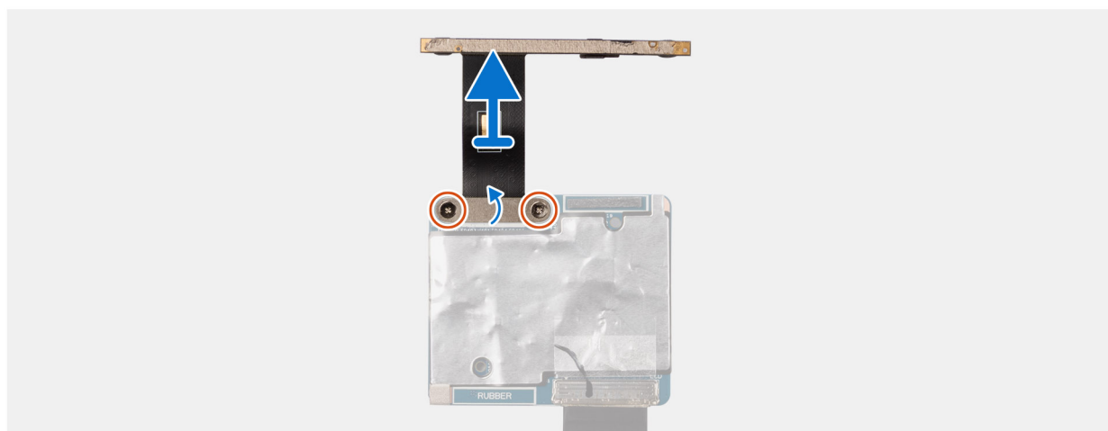
Figura 66. Removing the camera
