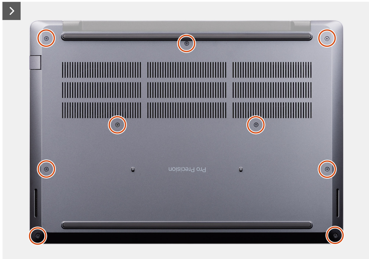
Figura 2. Loosen the captive screws
