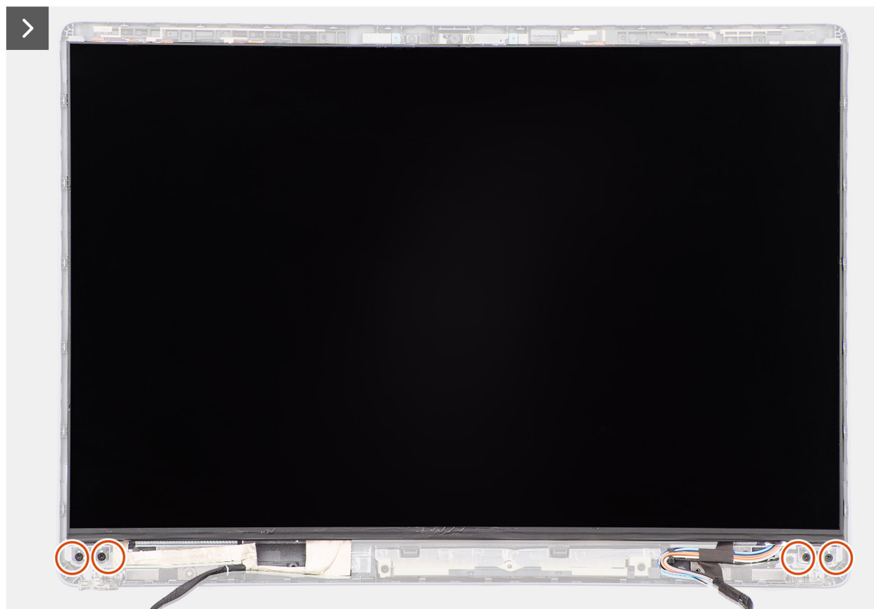
Figura 56. Removing the display panel
