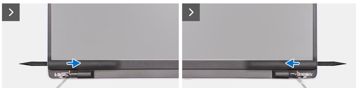
Figura 52. Removing the display bezel
