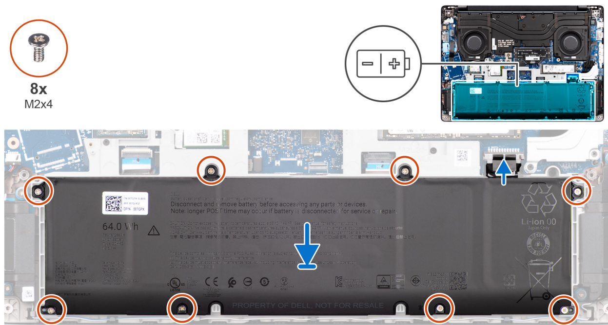
Figura 7. Installing the battery
