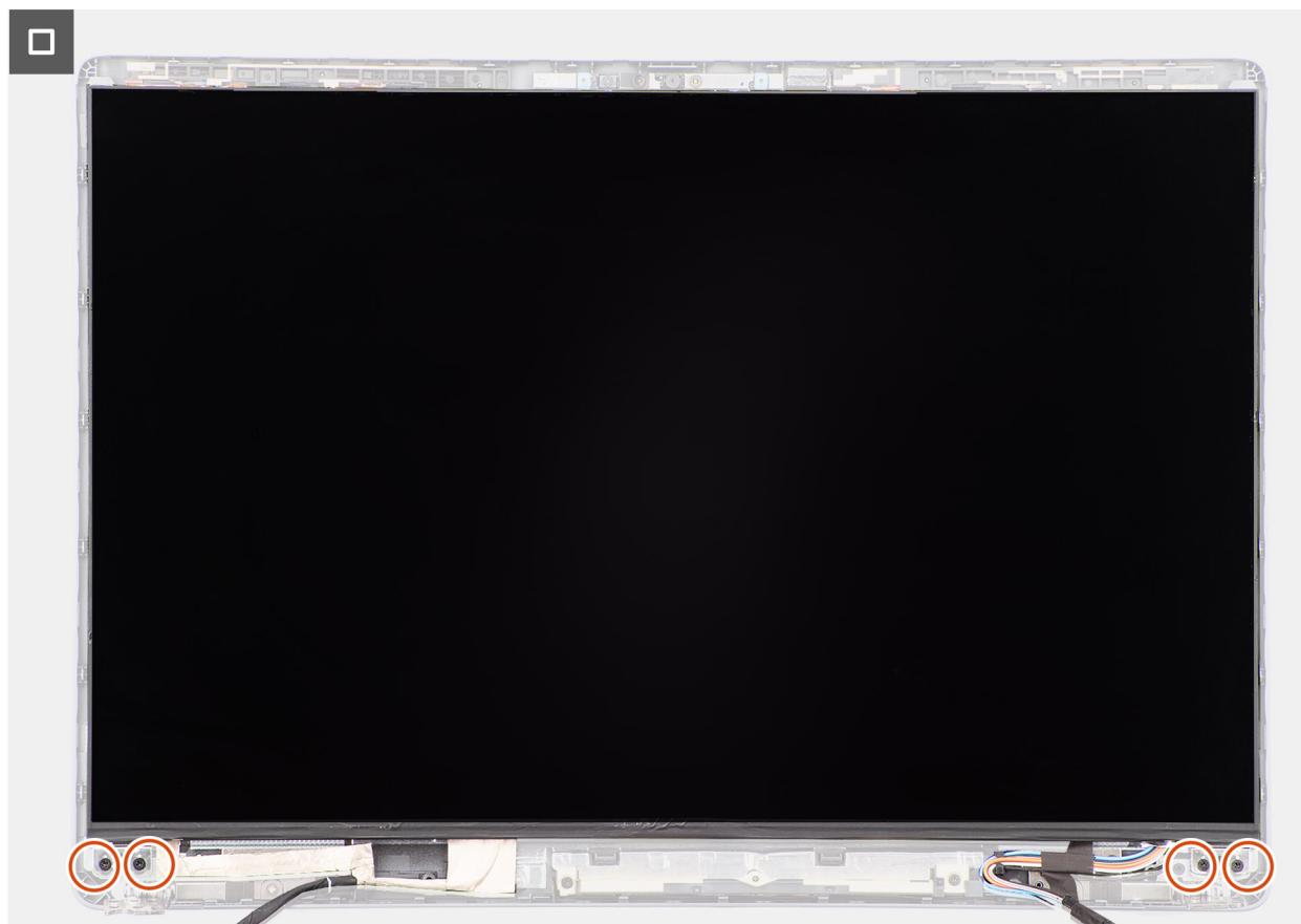
Figura 61. Installing the display panel
