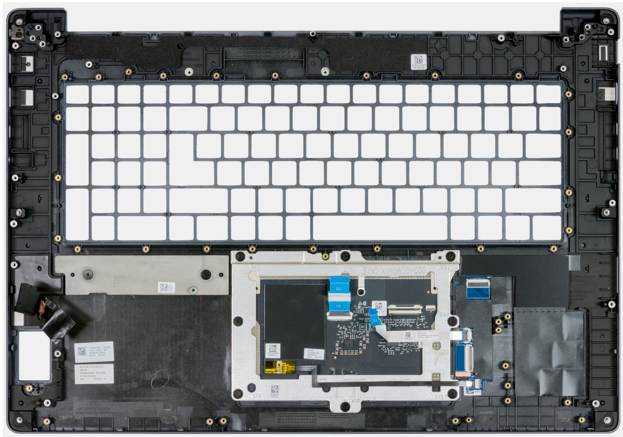
Figure 130. Assemblage du repose-poignets
