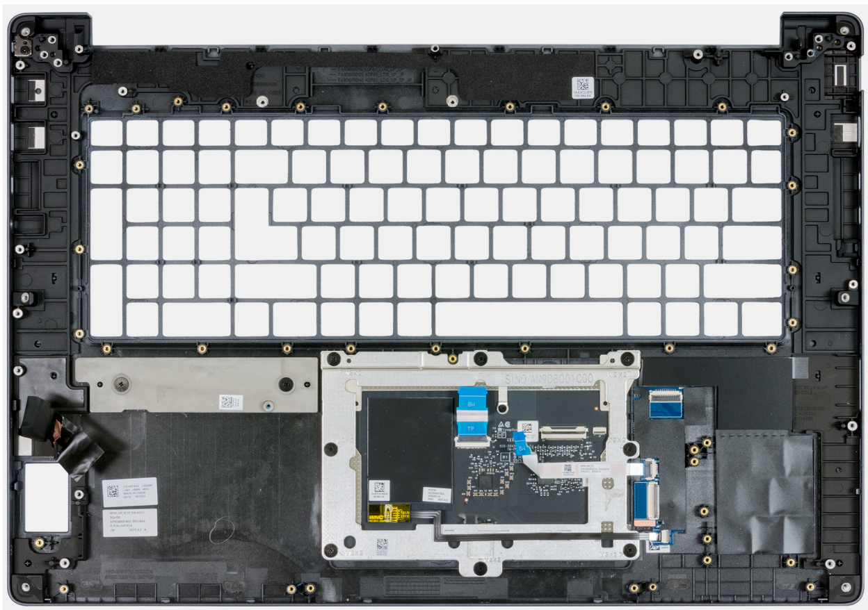
Figure 129. Assemblage du repose-poignets
