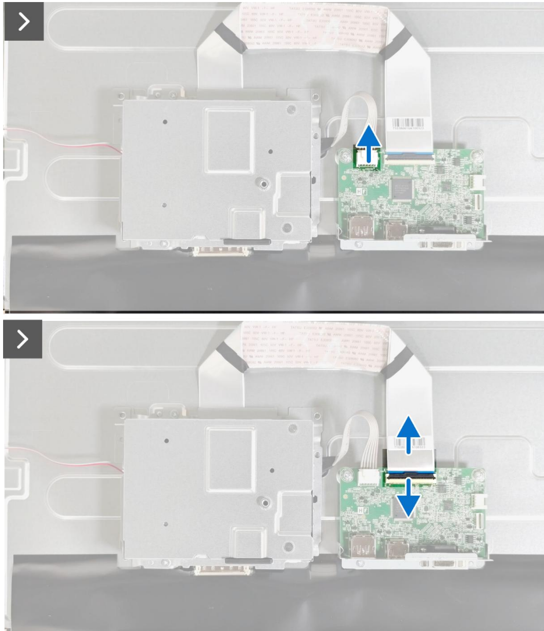
Figure 31. Removing the chassis assembly
