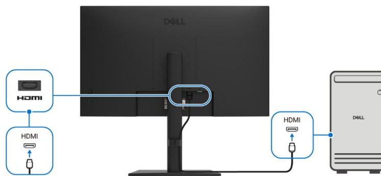
Figure 9. Connecting the HDMI cable
