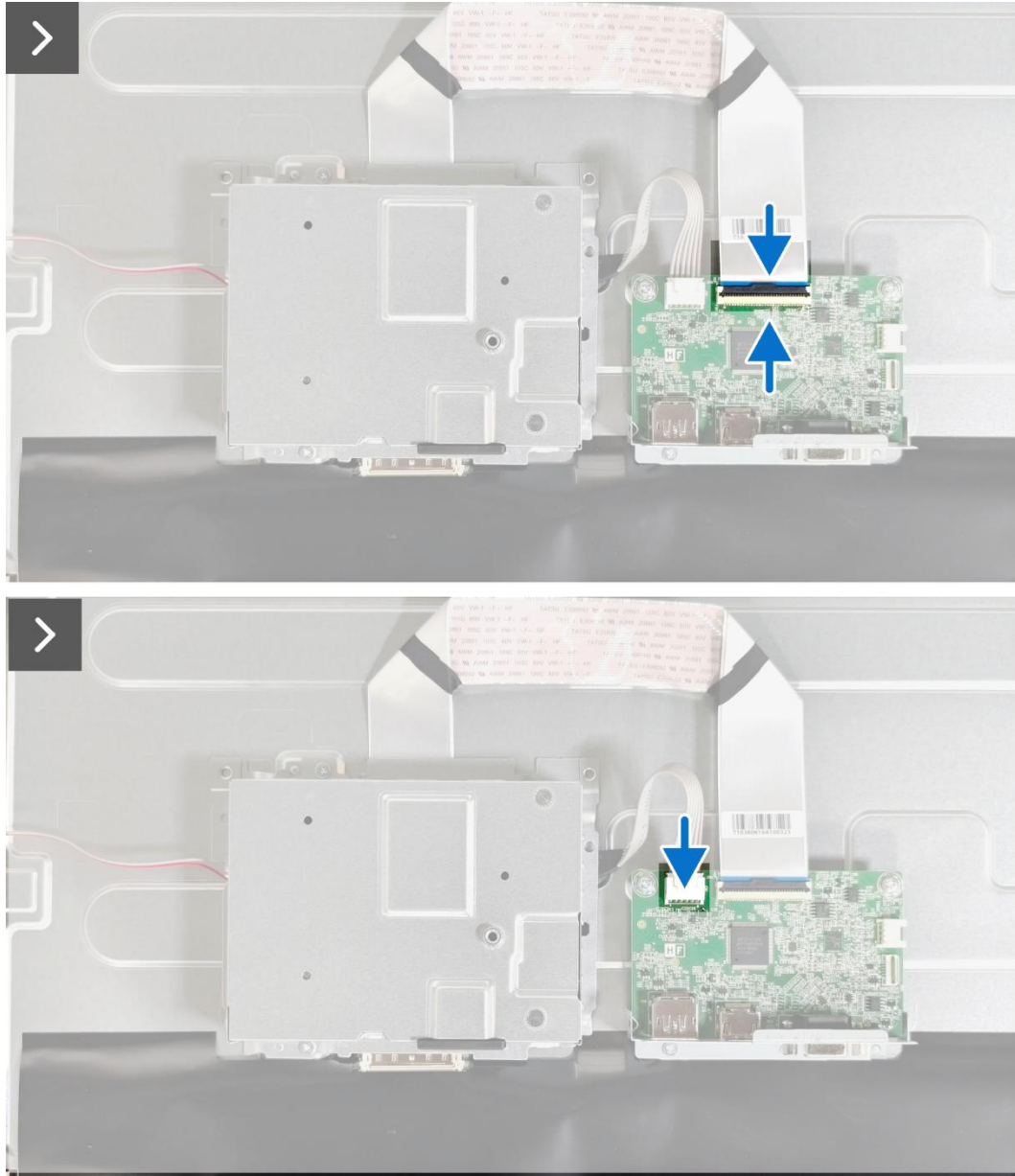
Figure 33. Installing the chassis assembly
