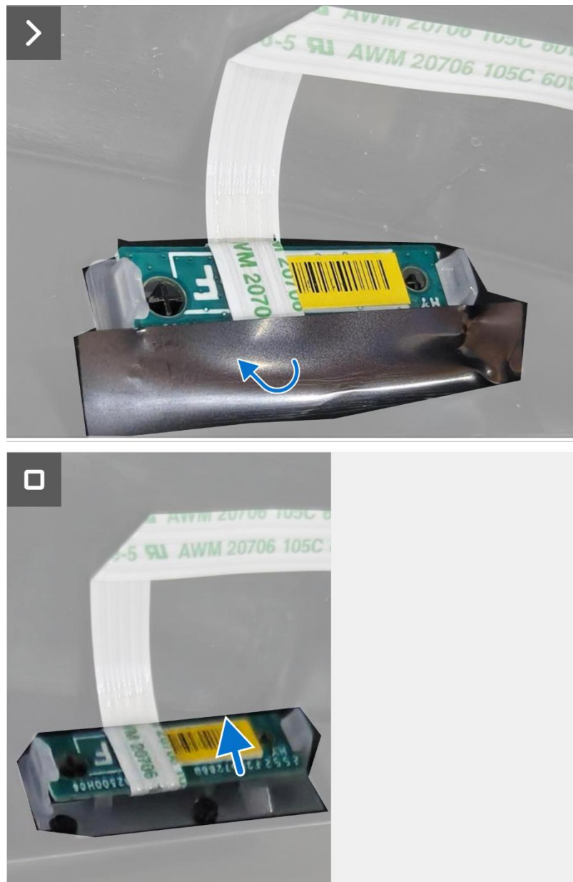
Figure 22. Removing the LED board
