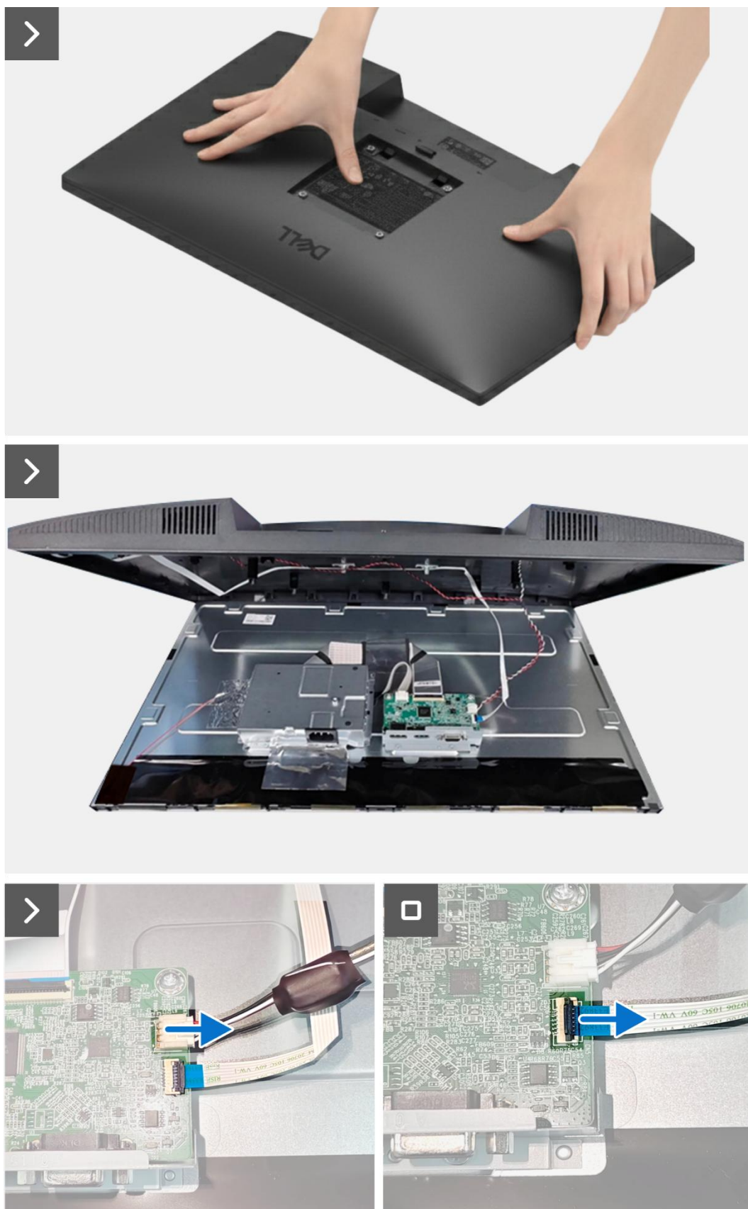
Figure 15. Removing the back cover
