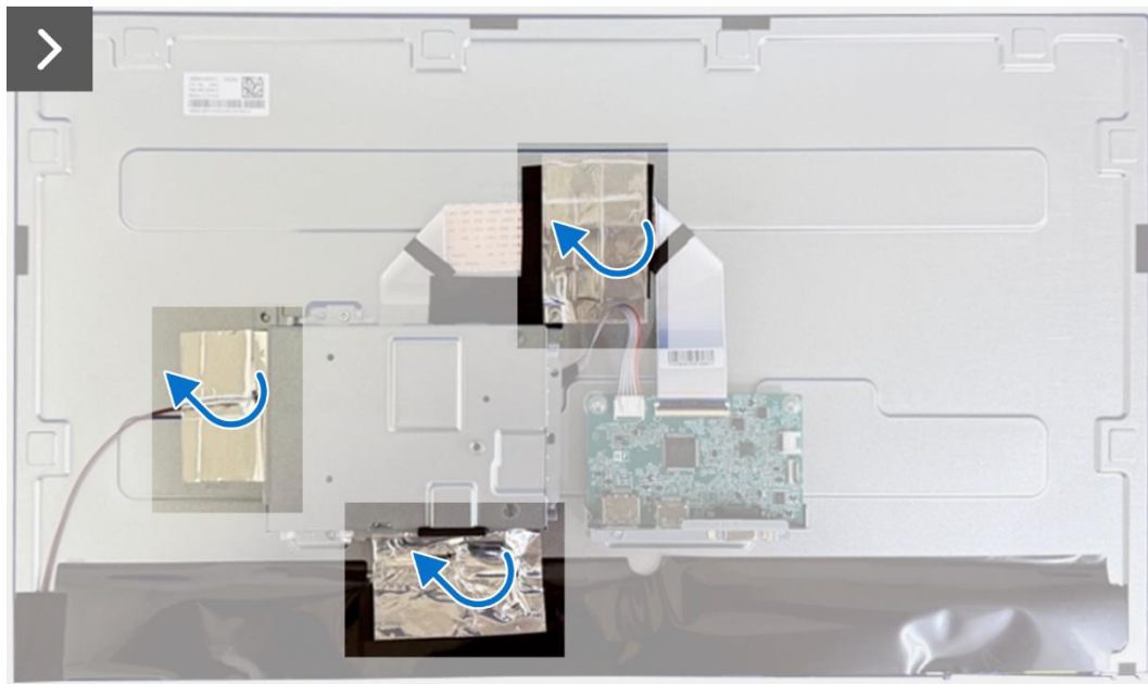
Figure 29. Removing the chassis assembly
