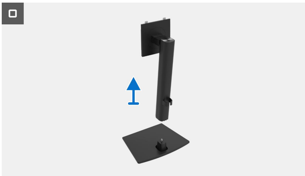
Figure 11. Removing the stand
