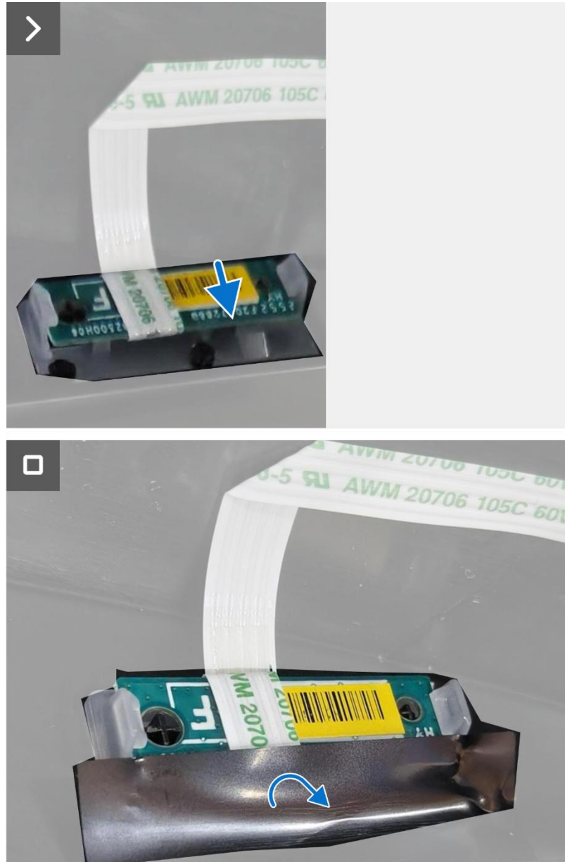
Figure 23. Installing the LED board
